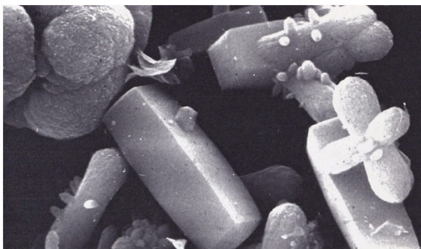
Figure 3.10. SEM of physical mixture of silicalite-2 and ZSM-48 synthesised at 130°C after 120 hours with an initial \text{OH}^-/\text{SiO}_2=0.10 .
