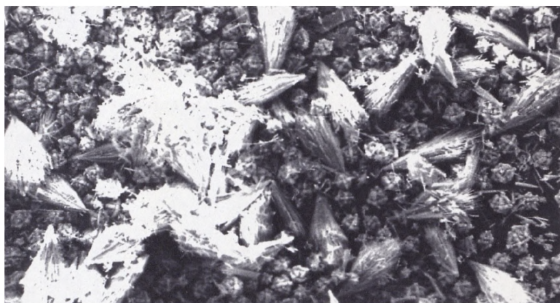
Figure 3.22b. Phases synthesised at 175°C after 35 days.
