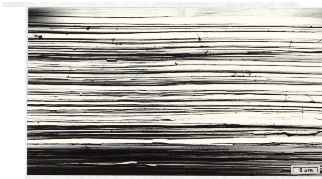
Fig.3.11 TEM micrograph of the replica for the unetched monofilament of Fibre A.
