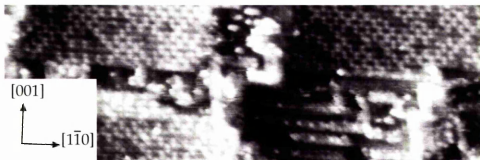
Figure 7.6: STM image ( 50 \text{ nm} \times 17 \text{ nm} ) of 0.7 ML of \text{Ca}/\text{TiO}_2(110) prepared by bulk segregation of calcium.
