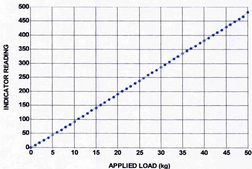
Figure (8.32) Load Cell Calibration 03 (1kg = 9.55)
