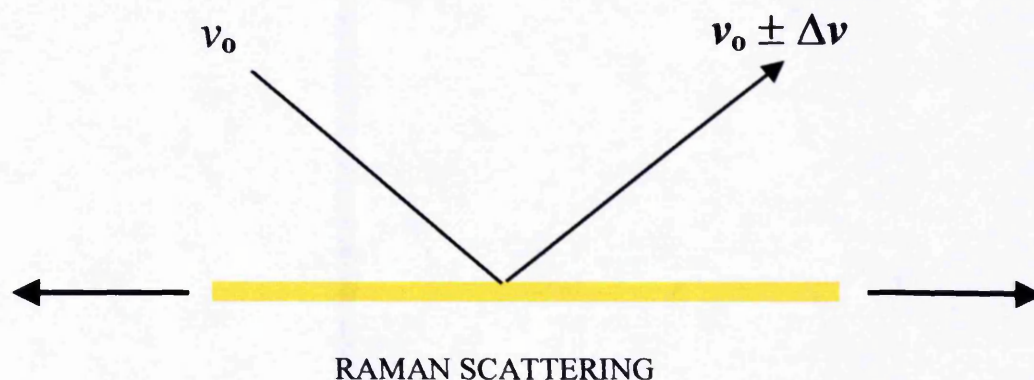
Figure (6.2) Schematic Diagram of the Raman Effect for a Fibre Subjected to Stress [76]
