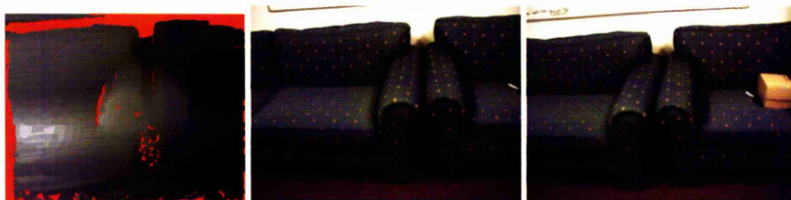
Figure 10.10: Depth map (left) generated from the pair of images (right) of a sofa and chair. The depth map is from the point of view of the middle image.
