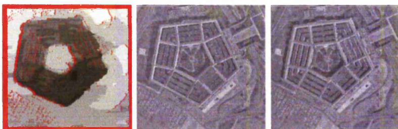
Figure 10.8: Disparity map (left) generated from the pentagon image pair (right).
