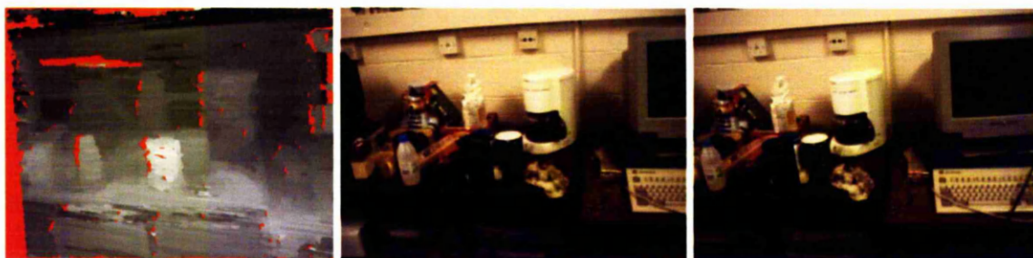
Figure 10.9: Depth map (left) generated from the pair of images (right) of a cluttered desk. The depth map is from the point of view of the middle image.
