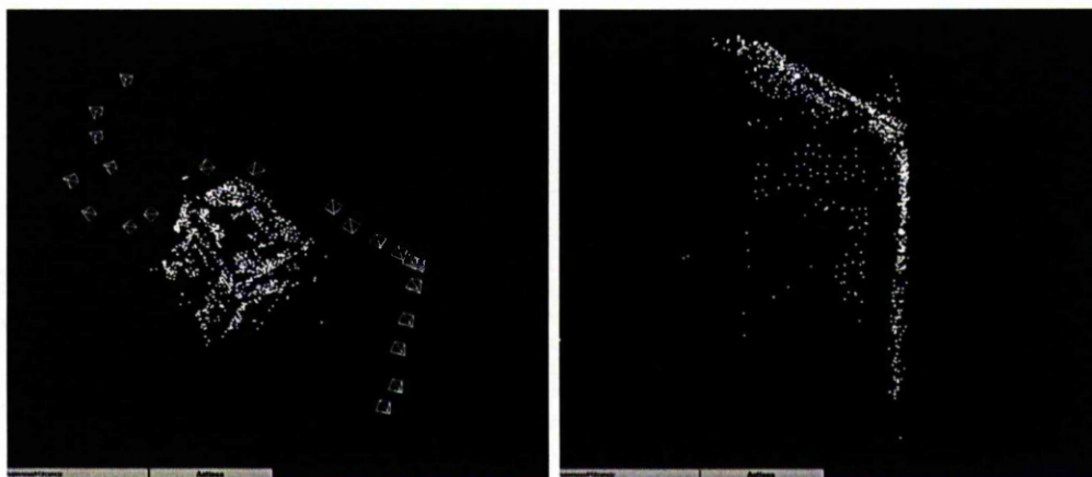
Figure 10.6: Two views of the sparse set of calibrated points and cameras generated from the box scene.
