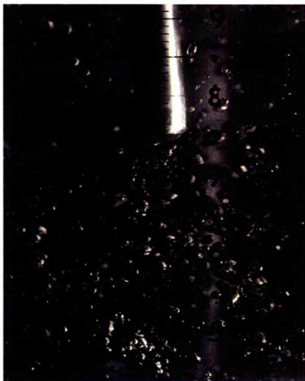
Figure 5-18: Gas bubbles in hot methanol sparged with ethylene at 10 barg
