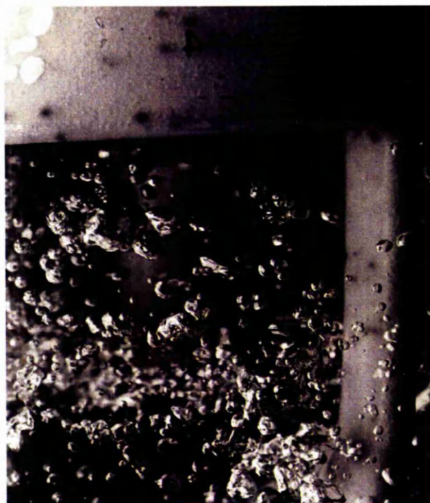
Figure 5-11: Water vapour bubbles in boiling water
