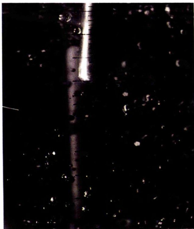
Figure 5-11: Water vapour bubbles in boiling water
