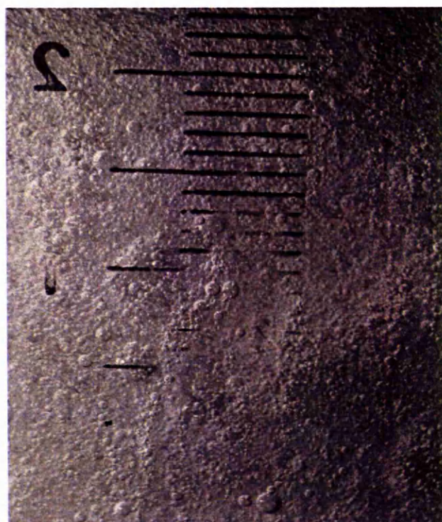
Figure 5-15: Gas bubbles in boiling aniline sparged with nitrogen
