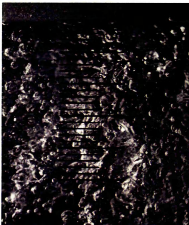
Figure 5-9: Gas bubbles in nitrogen sparged boiling acetic acid
