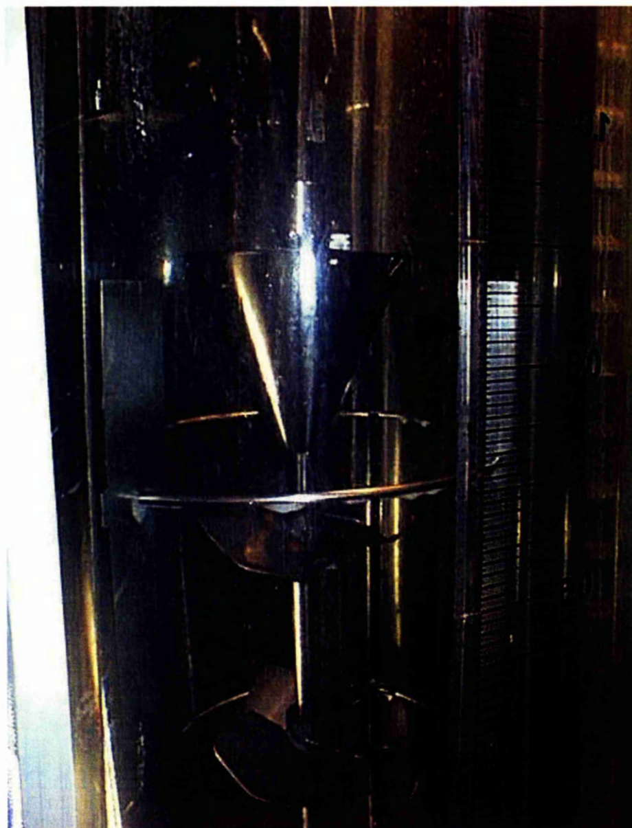
Figure 8-13: Dual A345 agitators with a 30° cone in the 0.61 m diameter vessel.
