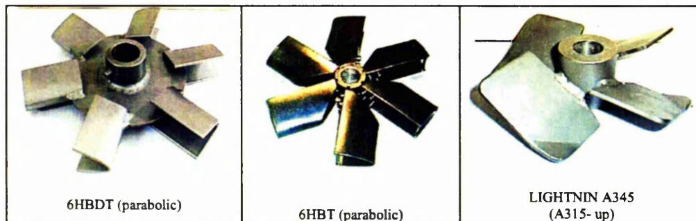
Figure 7-25: Agitators tested for solid suspension on the 0.286 m vessel
