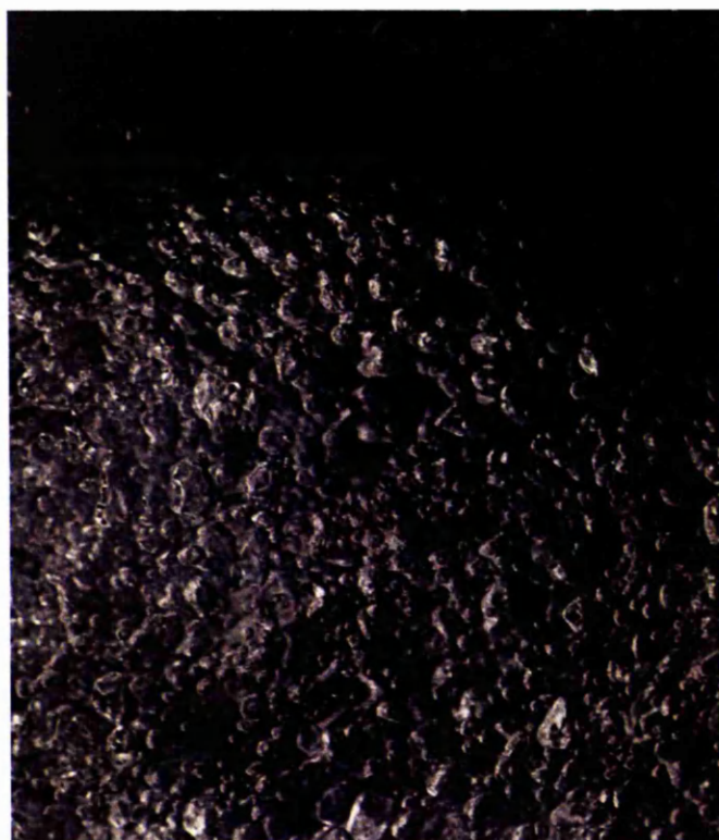
Figure 5-8: Nitrogen bubbles in cold acetic acid
