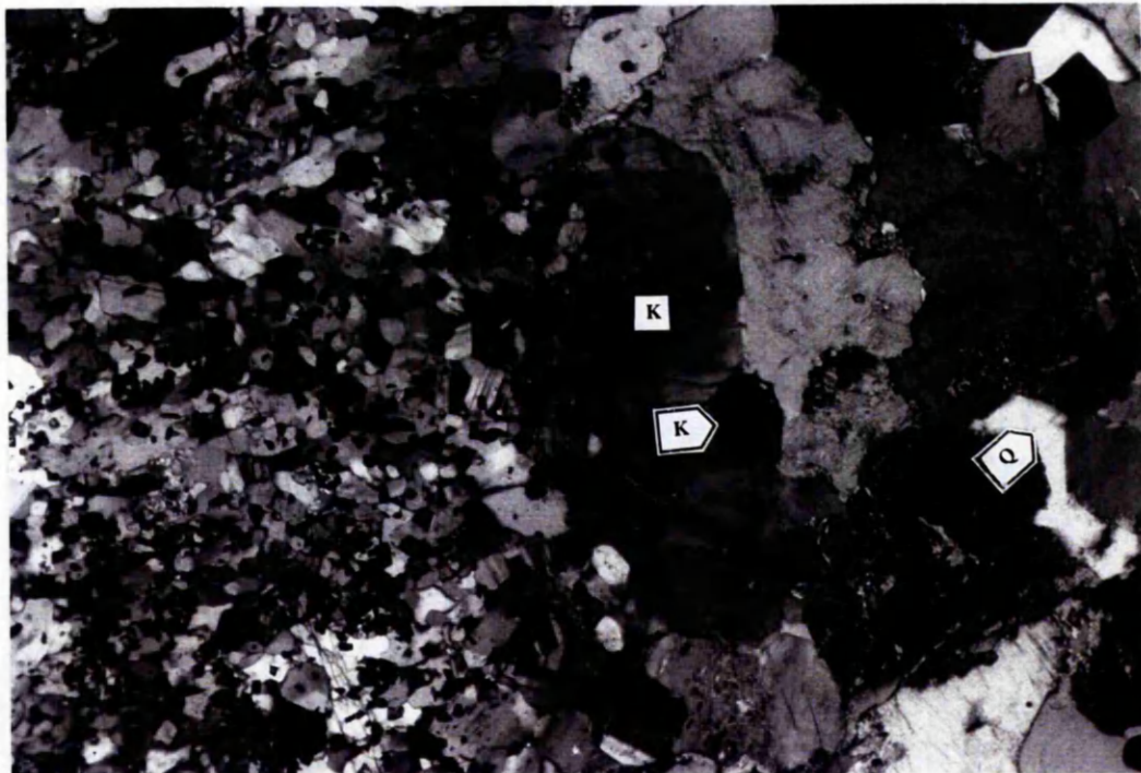
Plate 6.10 as above in XPL to show the interstitial-xenomorphic texture of quartz and euhedral to subhedral texture of K-feldspar.
