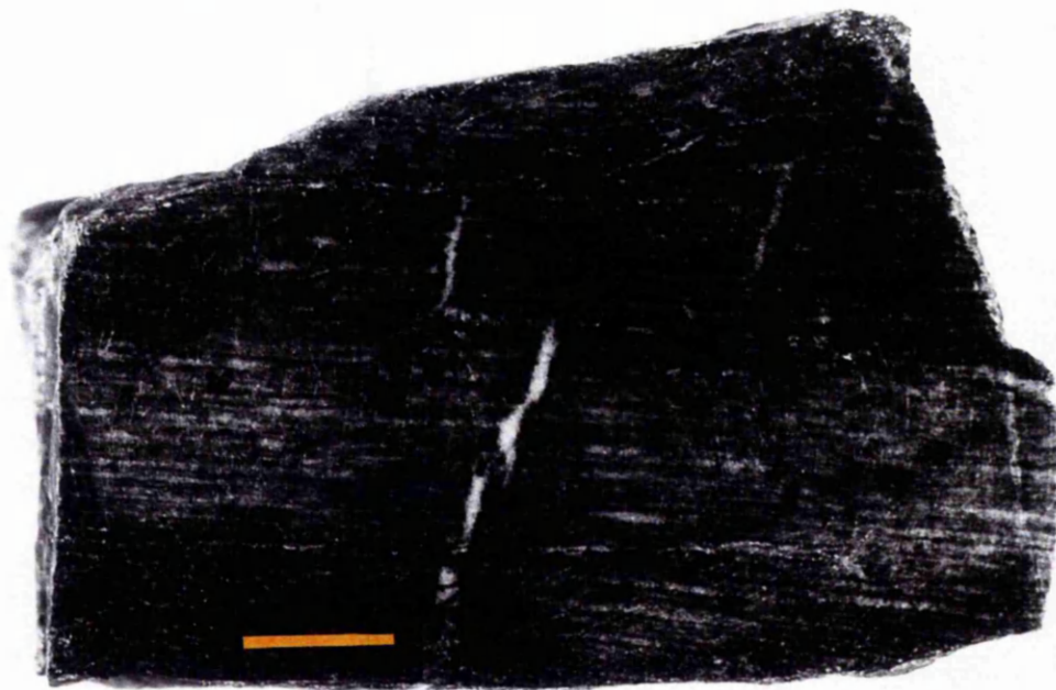
Plate 6.2 A cut and polished hand specimen of migmatite with pull-apart structure. One set of leucosomes are parallel to the former S_2 crenulation cleavage and the other set cut the crenulation. Dark spots on the rock surface shows cordierite-rich patches. The scale bar is 1 cm I ong.
