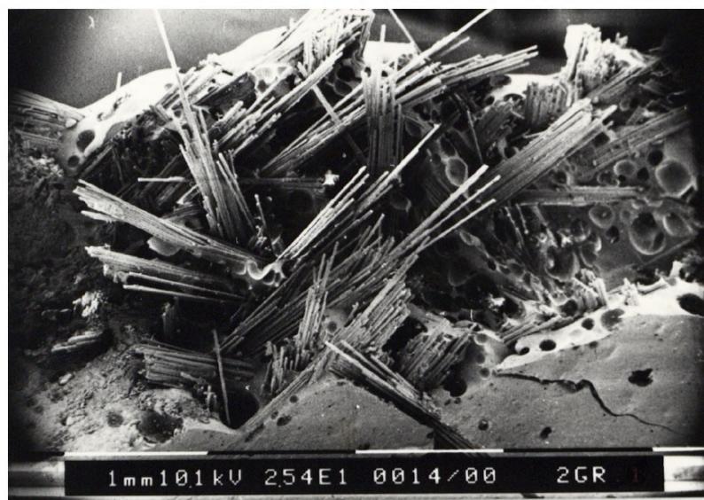
Figure 5.41 Fractography of SRIM composites of 2GR
