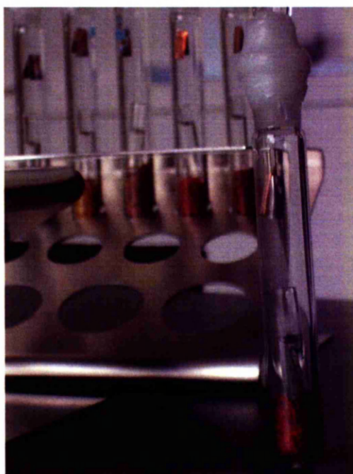
Figure 6.2.1. Thermal Oddy test setup
