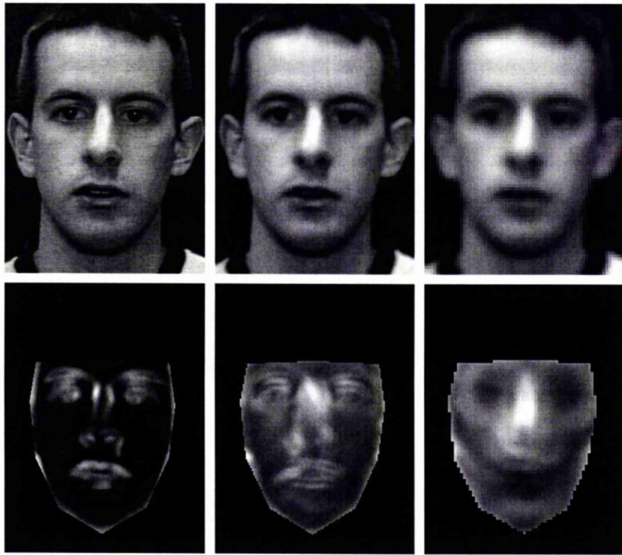
Figure 5.8: The saliency maps extracted from the first 3 levels of a Gaussian image pyramid (fine to coarse scale going from left to right). Bright regions are the most salient.
