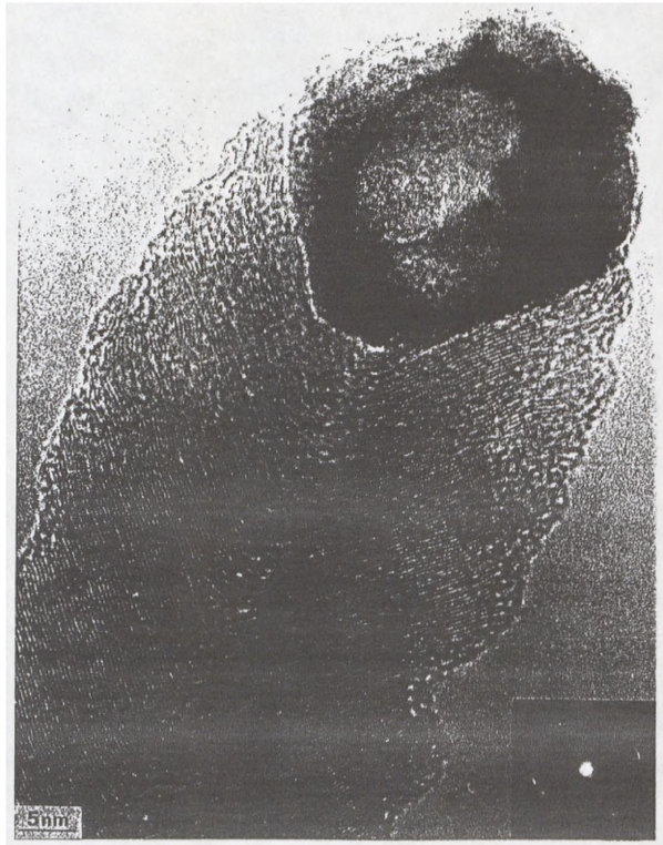
Fig.1.12(a) Structure of a full (true) carbon filament formed on Ni/Al 2 O 3 at 873 K [60]
