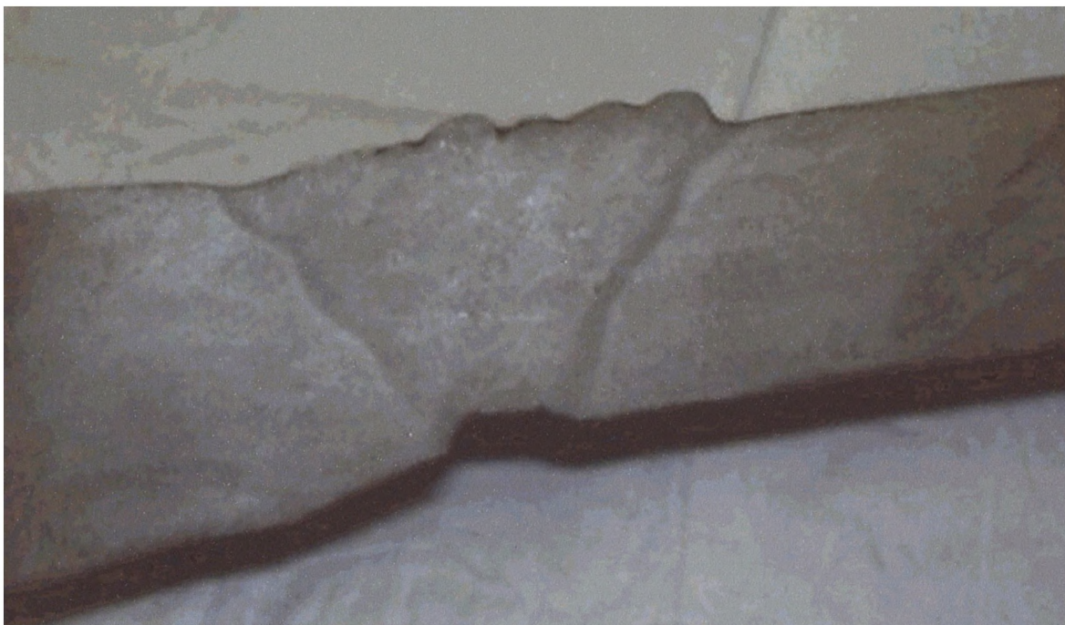
Figure 3.1 A cross-section of joint 3 of the Waveney Spoolpiece after polishing and etching.
