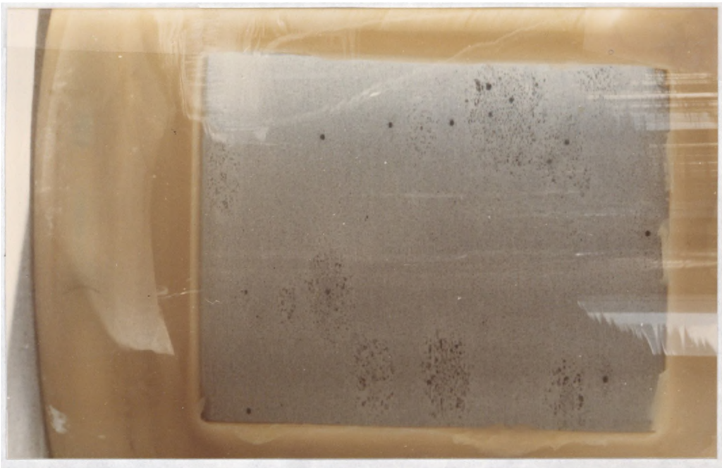
Plate 3.5 VAGH-N, 5 days in deaerated solution.
