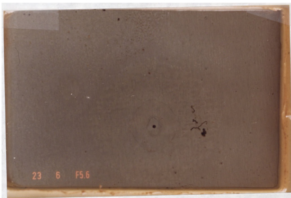
Plate 3.10 Acrylic A2 after 48 days immersion.
