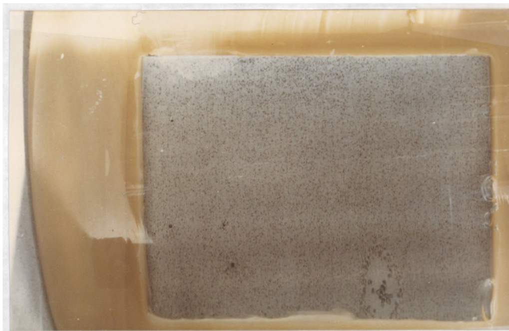
Plate 3.7 VMCH-N, 5 days in deaerated solution.
