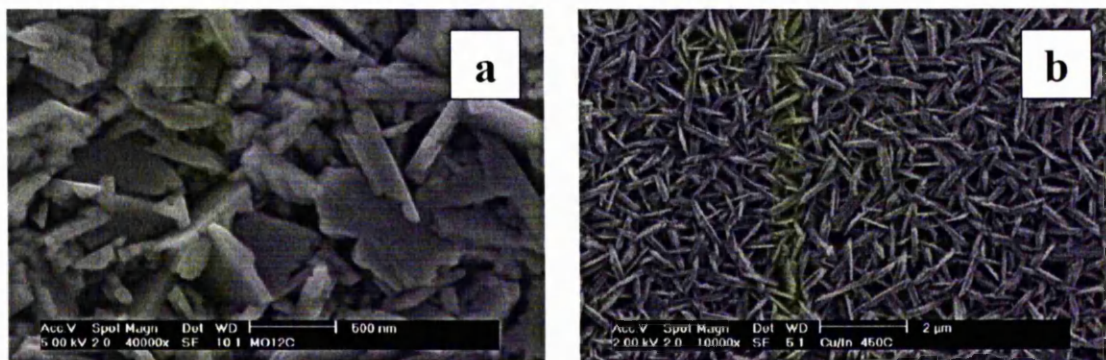
Figure 2.14 SEM images of CuInS 2 films deposited at (a) 350 °C and (b) 450 °C.
