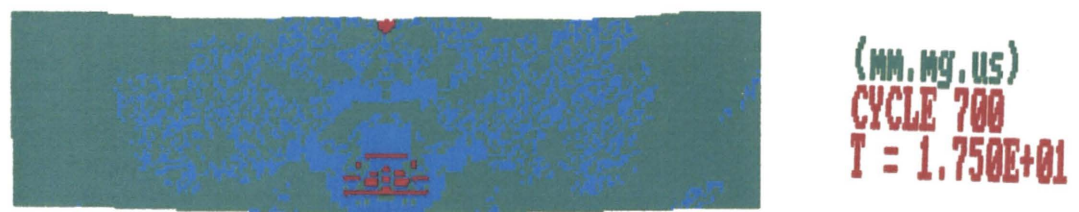
Fig. 12.20 Stress-wave Focussing Arrested Experimental Spall Compared with Simulation
