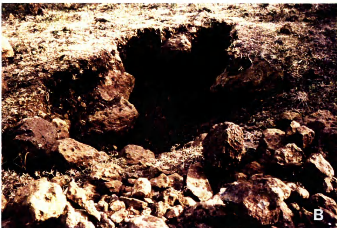
Figure 4.7 The residual soil and gravels on top of the basalt outcrop at Khao Lan Thom, Bo Phloi were dug out to wash for the corundum by the miner standing on the pit A ), and the boulders of basalts and a hole were left on the ground B ).
