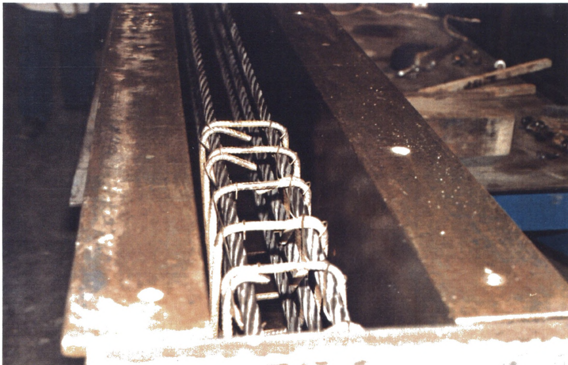
Plate 9.1- Test beam during construction, showing detail of stirrup location.
