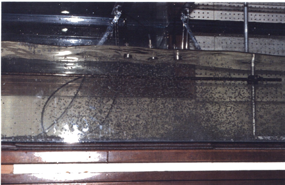
Plate 10.3- Linear array system with polystyrene beads in suspension used to simulate the effects of aggregate.
