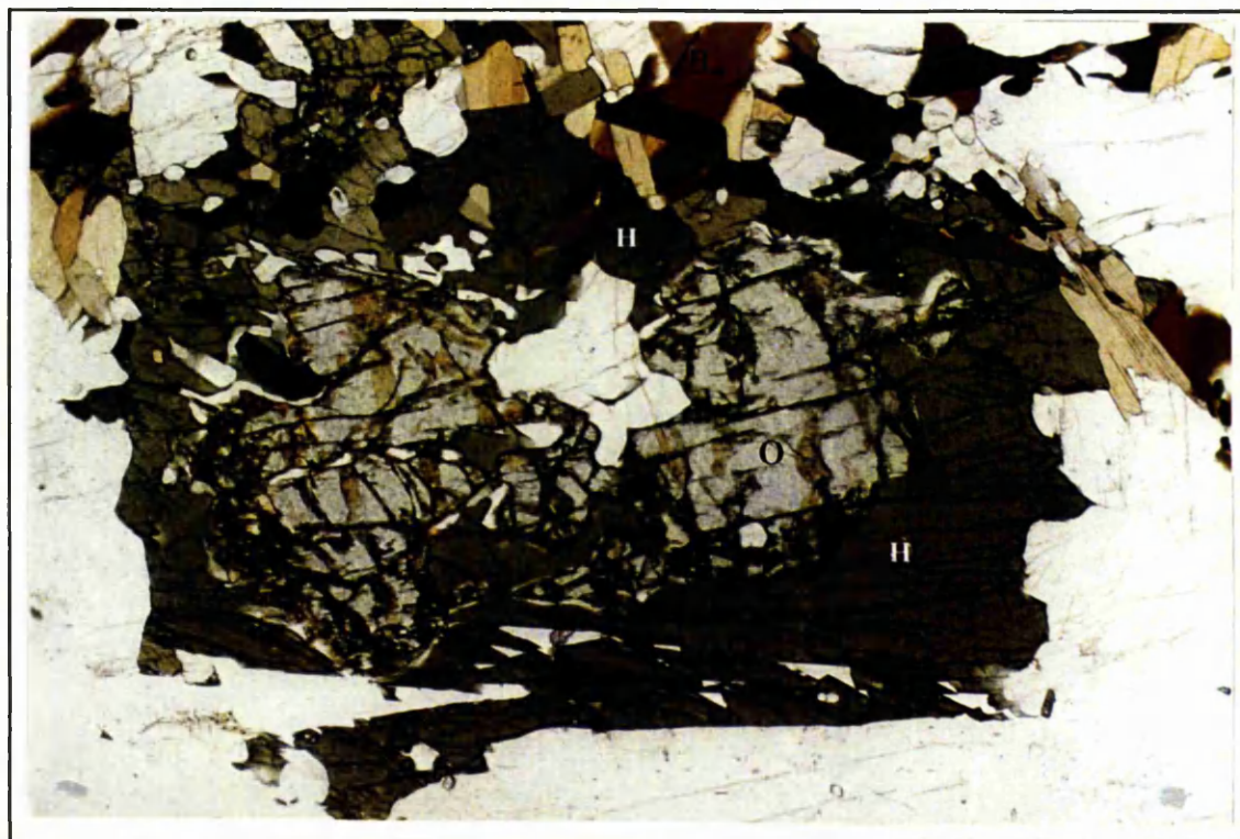
Plate 5.5.12 Photomicrograph from a garnet-hornblende tonalite (DD.CUM19). Weak-green pleochroic orthopyroxene (O), partially replaced by olive-green pleochroic hornblende (H). Red-brown biotite (B) is also present near the top of the plate. PPL, field of view 7.5 x 5 mm.
