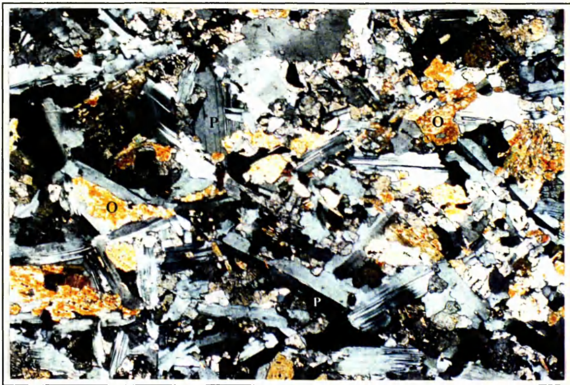
Plate 5.3.5 Photomicrograph of a micro-norite (H.BHQ4). Plagioclase (P) forms randomly oriented laths, with anhedral, interstitial orthopyroxene (O). XPL, field of view 3.75 x 2.5 mm.
