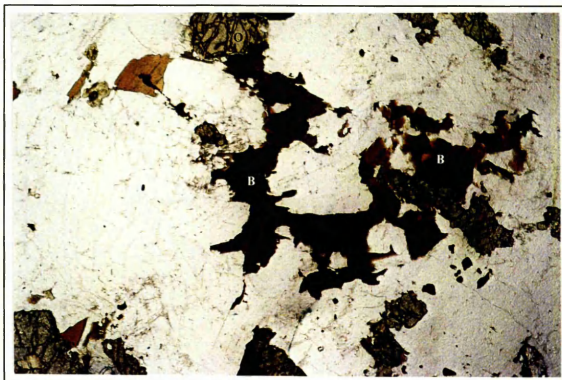
Plate 5.5.8 Photomicrograph from a cordierite norite (DD.BQ202ii). Poikilitic biotite (B) partially enclosing plagioclase. Pleochroic orthopyroxene (O) is also present. PPL, field of view 7.5 x 5 mm.
