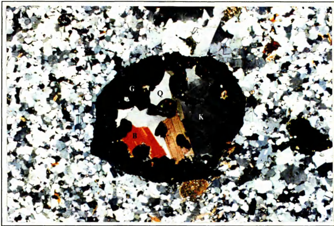
Plate 5.4.15 Photomicrograph of an orthopyroxene-cordierite hornfels (DDBQ201). A large atoll-type garnet (G) is 'filled' by coarse grained K-feldspar (K), quartz (Q) and biotite (B). The rock matrix is much finer grained and composed mainly of interlocking cordierite and plagioclase crystals, giving a good hornfelsic texture. XPL, field of view 7.5 x 5 mm.
