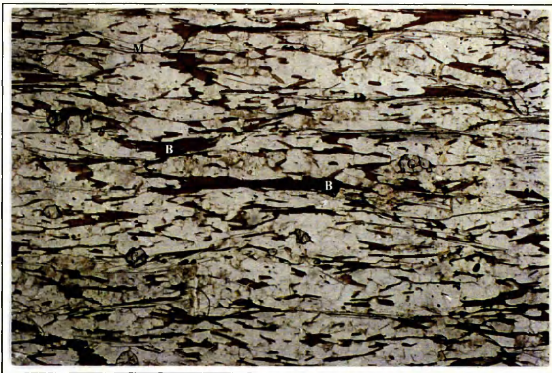
Plate 5.2.3 Photomicrograph of a garnet-mica schist (DD.SIN2). The brown pleochroic biotite (B) and muscovite (M) are foliated, with small garnets (G) evenly distributed across the section. PPL, field of view 7.5 x 5 mm.
