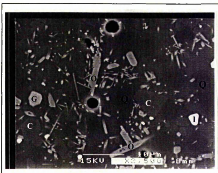
Plate 10.4.6 Backscattered electron image from run sample SIN2(900). The mineral phases visible are orthopyroxene, cordierite, ilmenite, G-garnet, and Q-quartz. The plagioclase and melt have similar atomic contrast and cannot be distinguished separately. The orthopyroxene is smaller than in CLAS112(900), forming elongate crystals and needles. The cordierite is euhedral and hexagonal in cross section.
