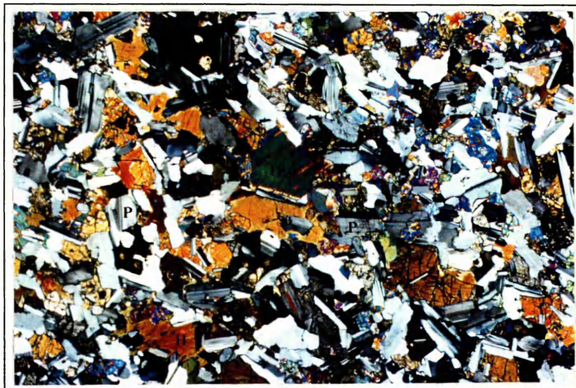
Plate 5.3.3 Photomicrograph of a biotite-hornblende dolerite (DD.H2). Plagioclase (P) forms randomly oriented, subhedral laths, with the high birefringence augite (A) mainly anhedral and interstitial. Hornblende (H) encloses smaller plagioclase laths. XPL, field of view 7.5 x 5 mm.
