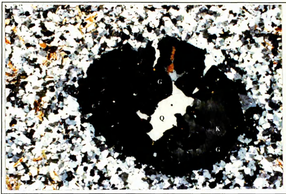
Plate 5.4.3 Photomicrograph of a cordierite-K-feldspar hornfels (H.COR4). Large atoll-type garnet (G), 'filled' with coarse grained K-feldspar (K) and quartz (Q). The matrix is composed mainly of fine-grained plagioclase and cordierite, which are intergrown to form a good granoblastic polygonal texture. XPL, field of view 7.5 x 5 mm.
