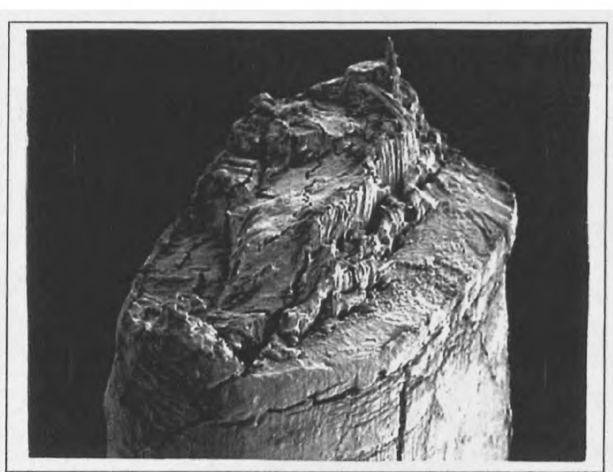
(x) Exposed Wool (208 hours) Tenacity: 7.5 cN/tex Extension: 2.3%
