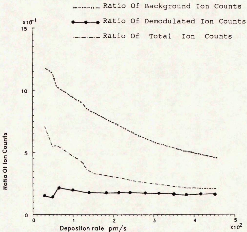
VARIATION OF THE RATIO OF BACKGROUND, DEMODULATED AND TOTAL ION COUNTS FOR  $Zn^+(m/e=33)$  OVER  $Zn^+(m/e=64)$  WITH THE DEPOSITION RATE (AT 2. mA Emmission Current)
