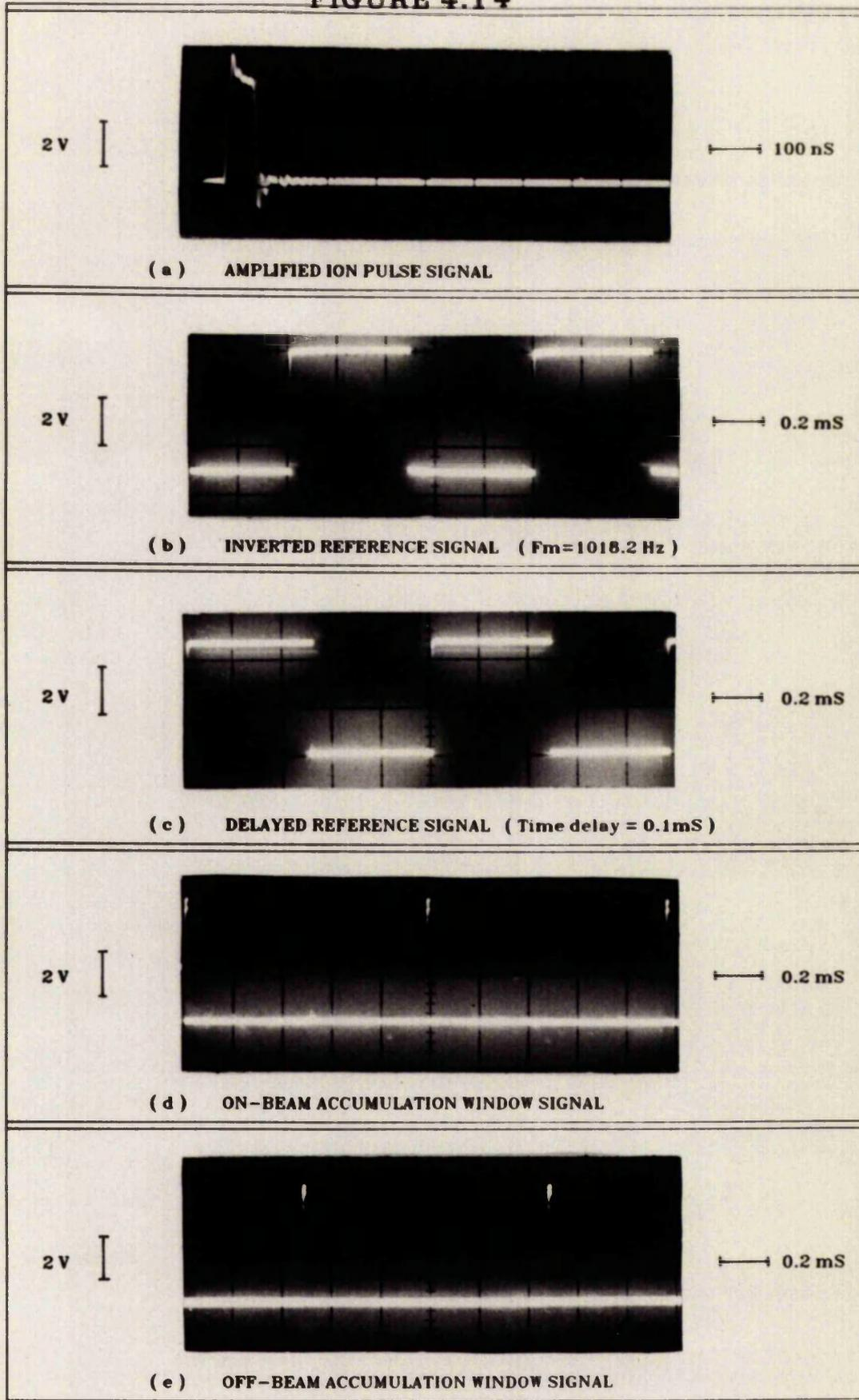
**DIAGRAM SHOWING THE OSCILLOSCOPE TRACES OF THE SIGNALS USED DURING THE TIME OF FLIGHT EXPERIMENTS.**
