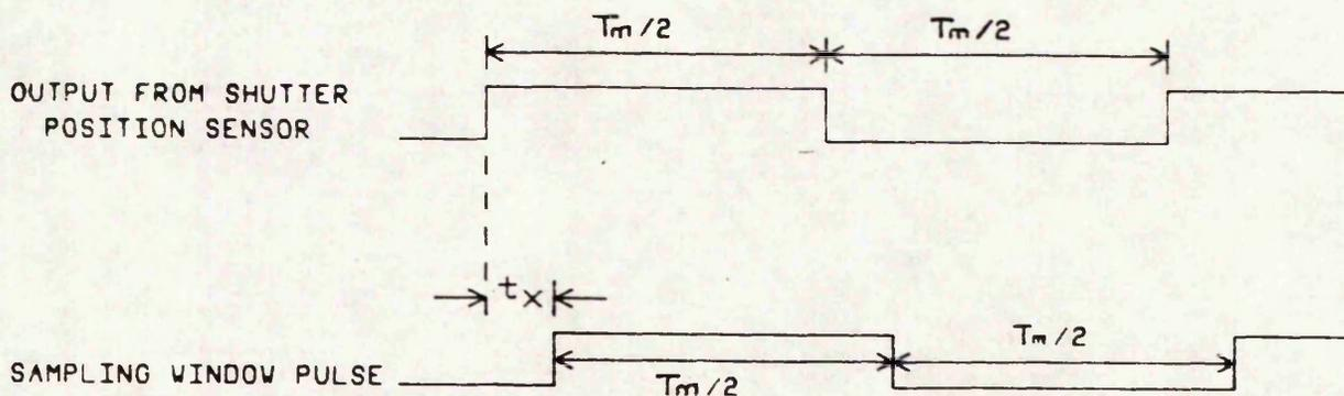
DIAGRAM SHOWING THE SIGNALS USED FOR INTEGRATED ION ARRIVAL DATA ACQUISITION USING A TIME WINDOW EQUAL TO  $T_m/2$
