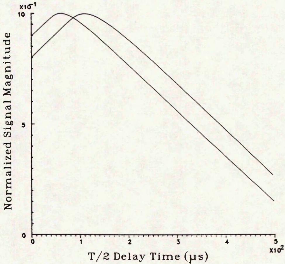
CALCULATED INTEGRATED ION ARRIVAL CURVES USING
