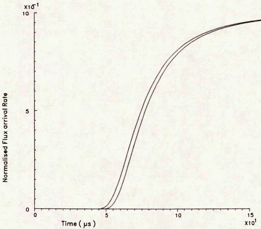
FIGURE SHOWING THE TIME LEAD INDUCED BY THE INTEGRATION OVER A  $6.4 \mu\text{s}$  WINDOW FOR  $\text{Se}^+$  (a.m.u=80) AT 900 CELSIUS
