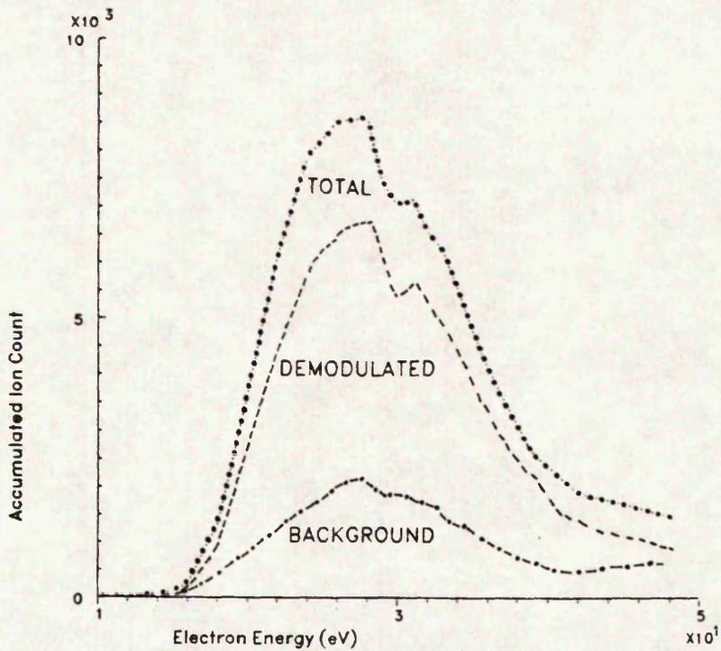
APPEARANCE POTENTIAL CURVES OF TOTAL, DEMODULATED AND BACKGROUND ION COUNTS FOR  $\text{Se}^+$  ( $m/e=80$ ) AT 900 CELSIUS
