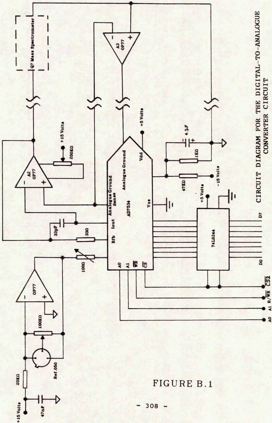
CIRCUIT DIAGRAM FOR THE DIGITAL-TO-ANALOGUE CONVERTER CIRCUIT
