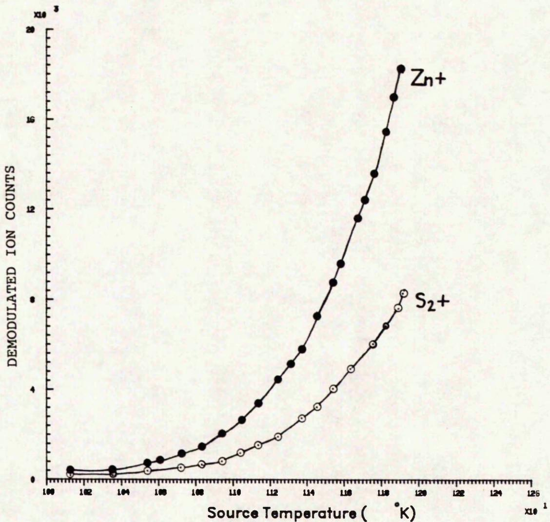
VARIATION OF THE INTENSITY OF  $Zn^+$  AND  $S_2^+$  NUMBER DENSITY AS A FUNCTION OF THE ABSOLUTE SOURCE TEMPERATURE
