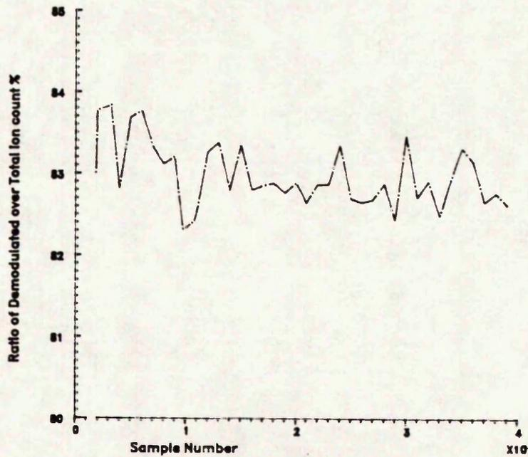
RATIO OF DEMODULATED OVER TOTAL ION COUNTS FOR  $SE^+$  IONS ( $m/e=80$ )
