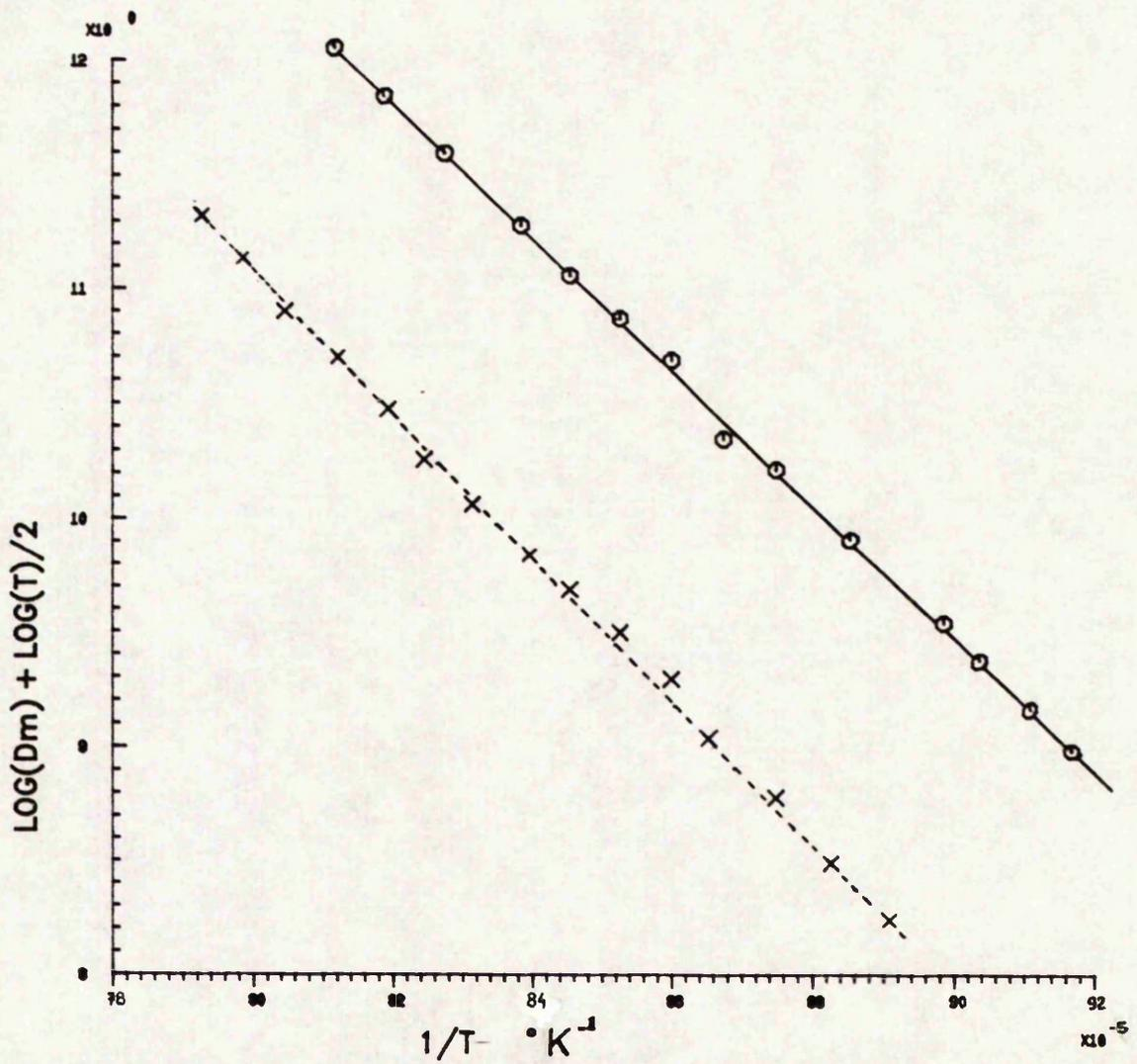
GRAPH OF  $\text{LOG}(D_m) + (\text{LOG}(T))/2$  vs THE RECIPROCAL OF ABSOLUTE TEMPERATURE FOR ZnS (+) AND ZnSe (o).
