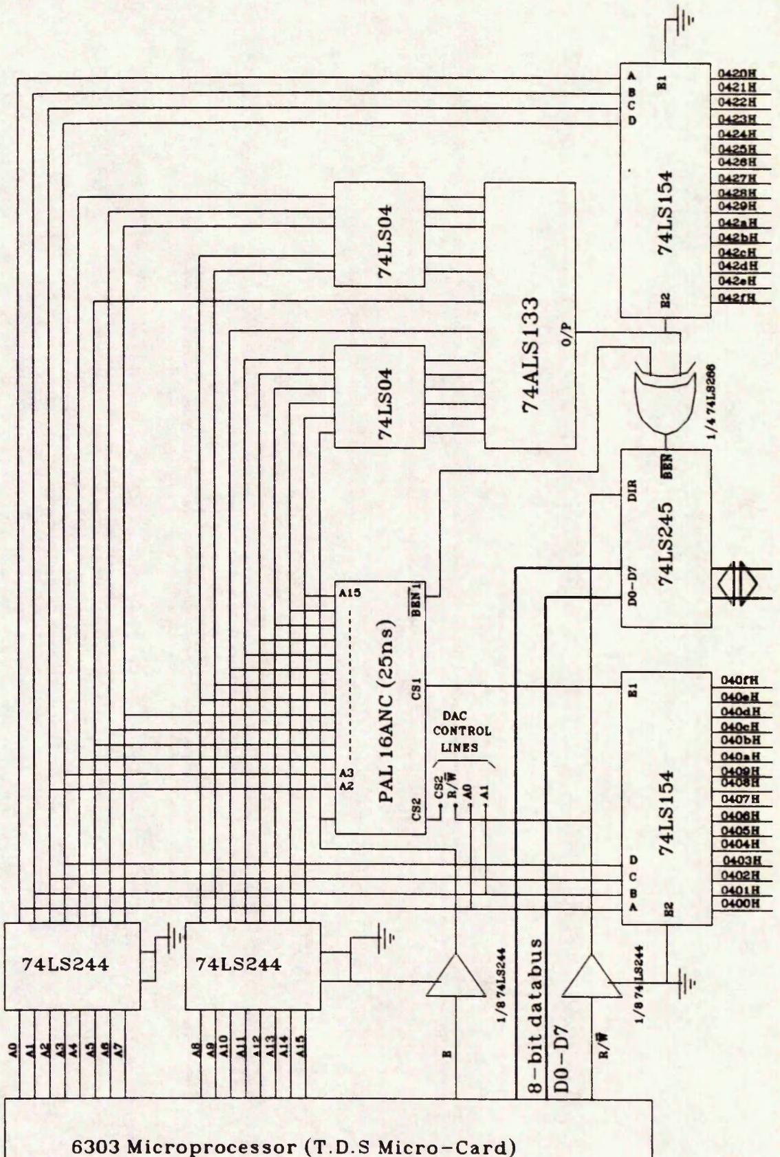
A programmable logic array device type PAL16ANC with a delay time less than 25 ns has been used to produce the following signals:
