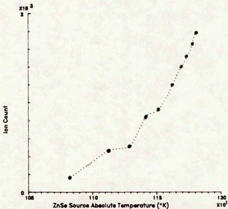
CALCULATED PROFILE VARIATION FOR THE ION COUNT ON Se + WITH THE ABSOLUTE TEMPERATURE OF THE ZnSe SOURCE
