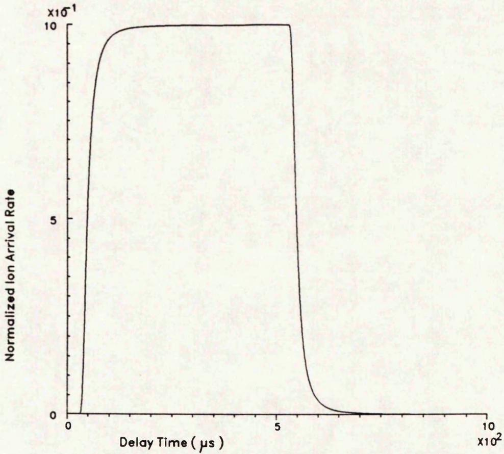
THEORETICAL ION ARRIVAL CURVE FOR SULPHUR ( S+ ) AT A MODULATION FREQUENCY OF 1 KHZ AND A TEMPERATURE OF 1000°C
