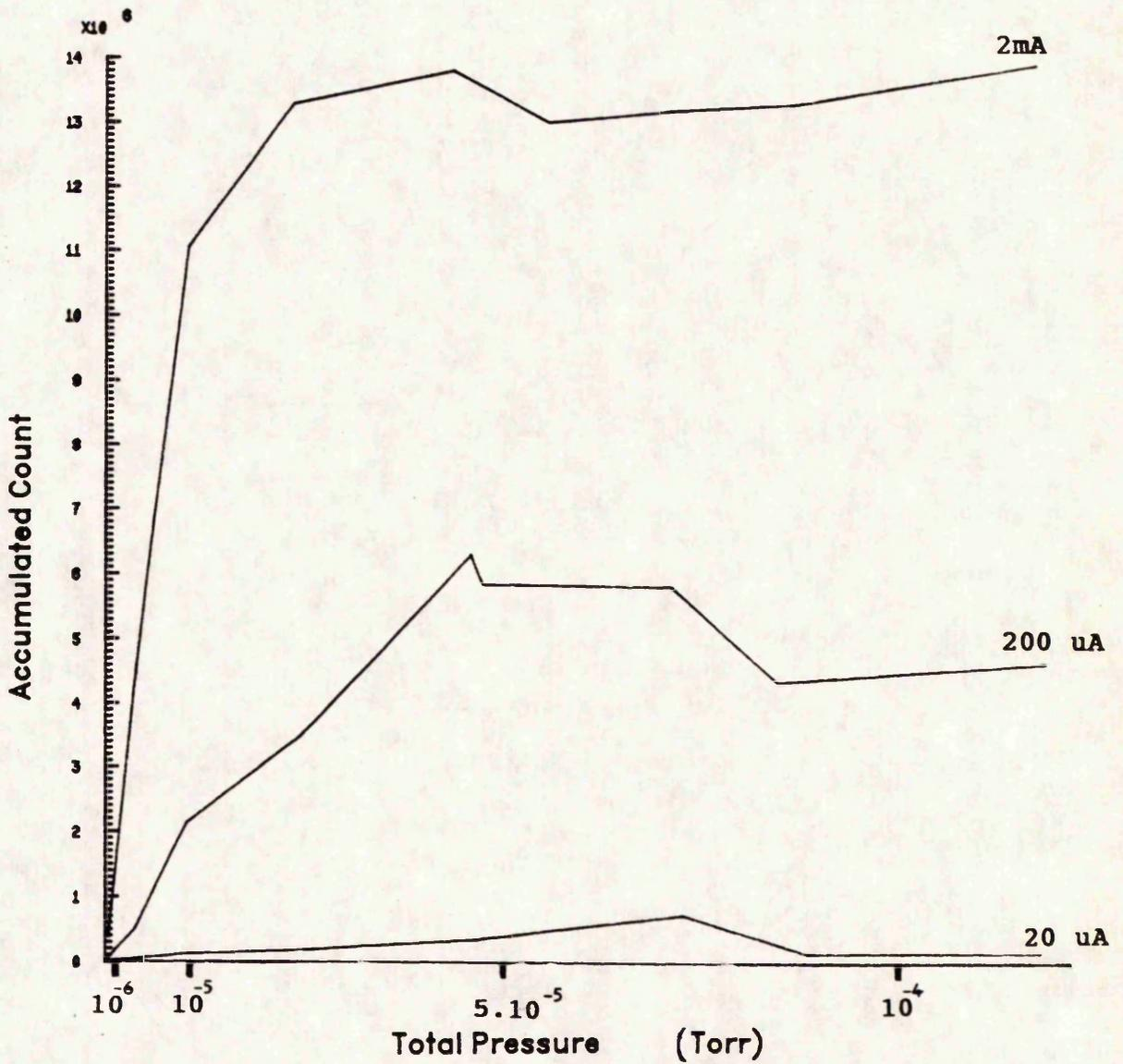
VARIATION OF  $N_2^+$  (m/e=28) ION COUNT WITH THE UHV SYSTEM TOTAL PRESSURE
