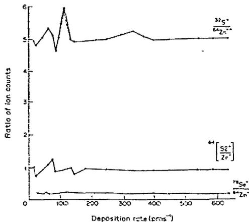
Figure 4. Ratios of ion species concentrations during the deposition of ZnS and of ZnSe.
