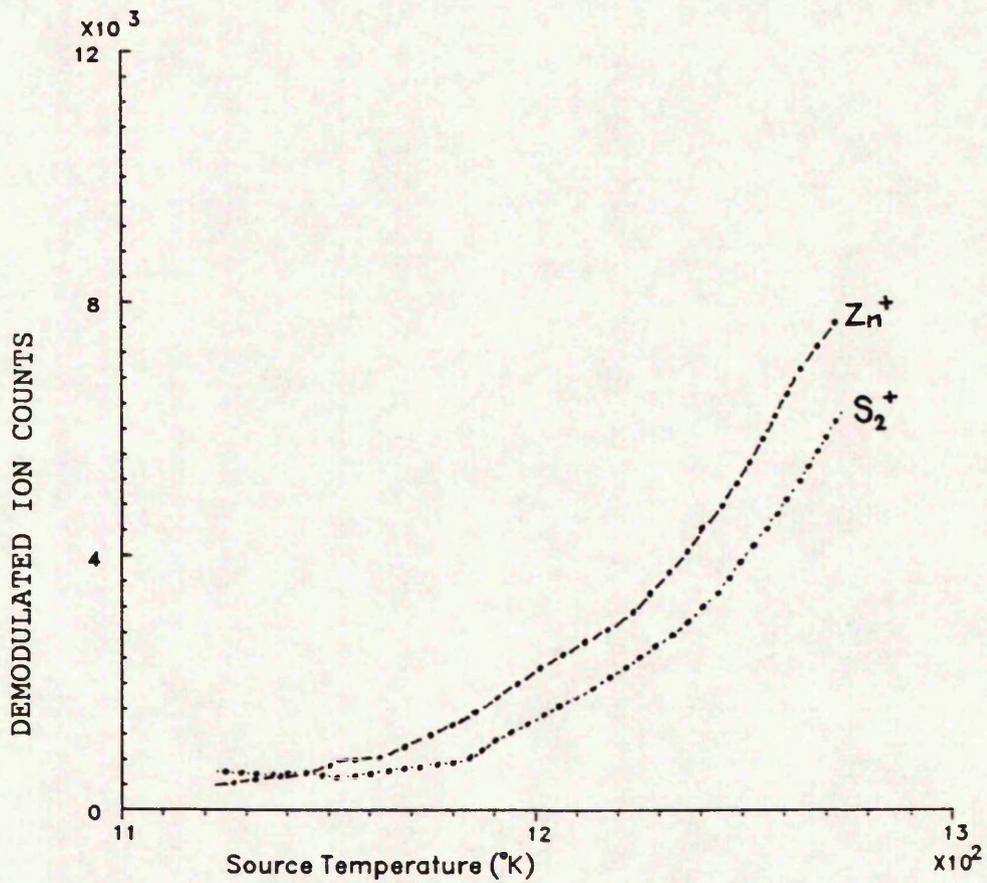
VARIATION OF S<sub>2</sub><sup>+</sup> AND Zn<sup>+</sup> ION COUNTS ( $m/e=64$ ) WITH THE ABSOLUTE SOURCE TEMPERATURE (MEASUREMENTS MADE USING EQUILIBRIUM SOURCE TEMPERATURES)
