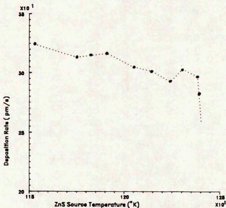
VARIATION FOR THE TOTAL DEPOSITION RATE WITH THE ZnS SOURCE TEMPERATURE DURING THE ZnS-ZnSe FILM GROWTH EXPERIMENT
