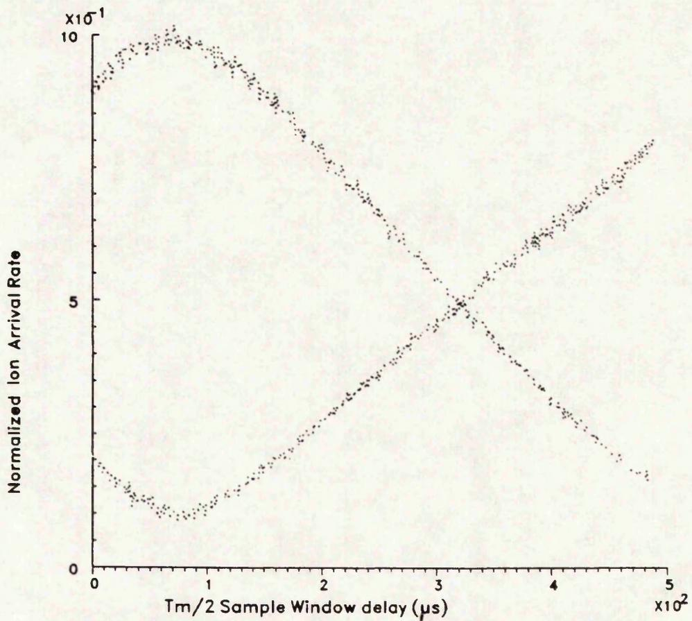
ALTERNATIVE REPRESENTATION FOR THE PRACTICAL INTEGRATED ION ARRIVAL DATA FOR  $\text{Zn}^+$  AT  $F_m = 1018.2 \text{ Hz}$  AND  $9.25 \text{ CELSIUS}$
