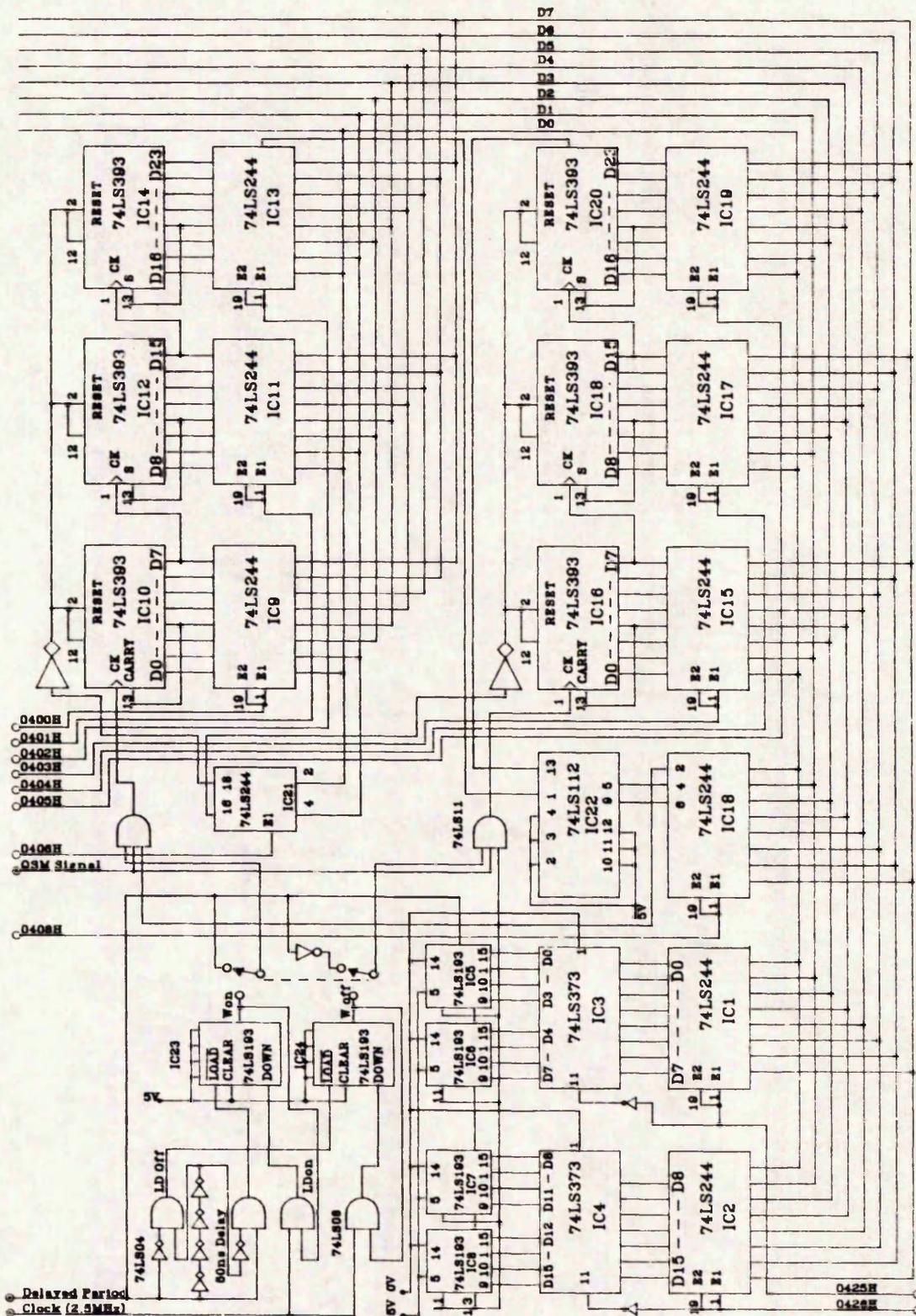
CIRCUIT DIAGRAM OF THE MASS SPECTROMETER ION PULSE COUNTING CIRCUIT
