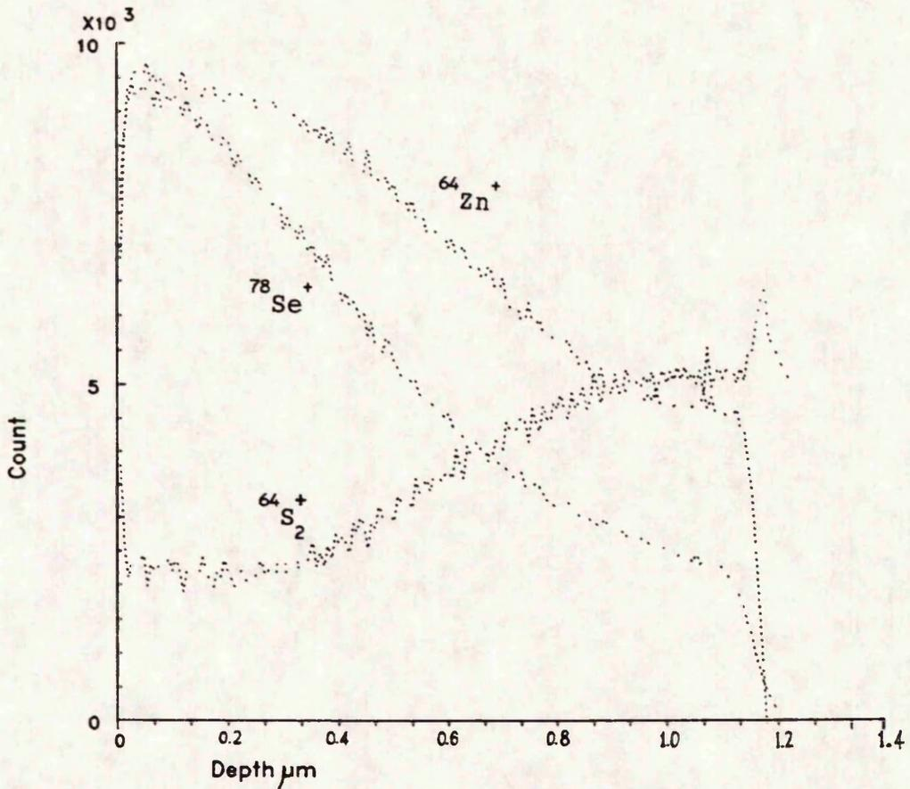
POSITIVE SIMS PROFILE FOR A ZINC SULPHOSELENIDE FILM INCLUDING  $\text{Zn}^+$  AT  $m/e=64$ ,  $\text{S}_2^+$  AT  $m/e=64$  AND  $\text{Se}^+$  AT  $m/e=78$
