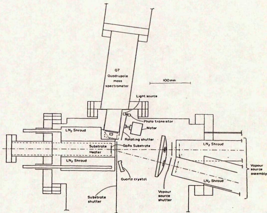
Figure 1. Cross-section of the ZnS-ZnSe deposition system.
