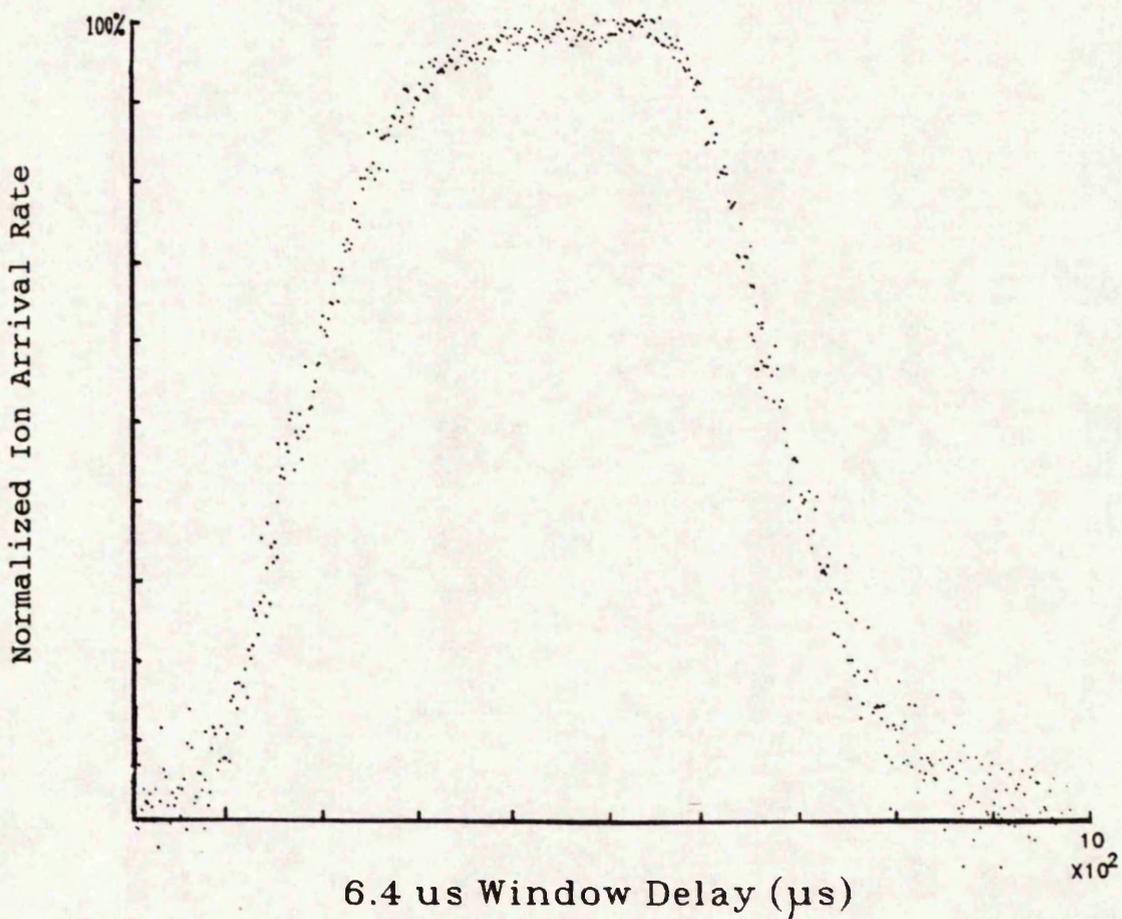
PRACTICAL ION ARRIVAL CURVE OBTAINED FOR Se+ AT A MODULATION FREQUENCY OF 1018.2 Hz, T=900 Celsius.
