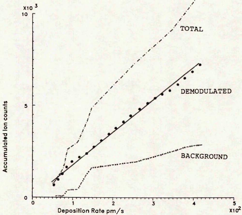
VARIATION OF  $S^{2+}$  ( $m/e=64$ ) ION COUNTS WITH THE TOTAL DEPOSITION RATE
