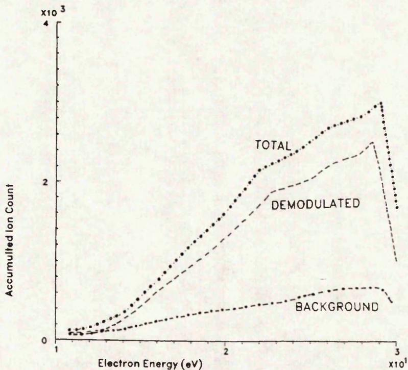
APPEARANCE POTENTIAL CURVES OF TOTAL, DEMODULATED AND BACKGROUND ION COUNTS FOR  $\text{Se}^{2+}$  ( $m/e=160$ ) AT 900 CELSIUS
