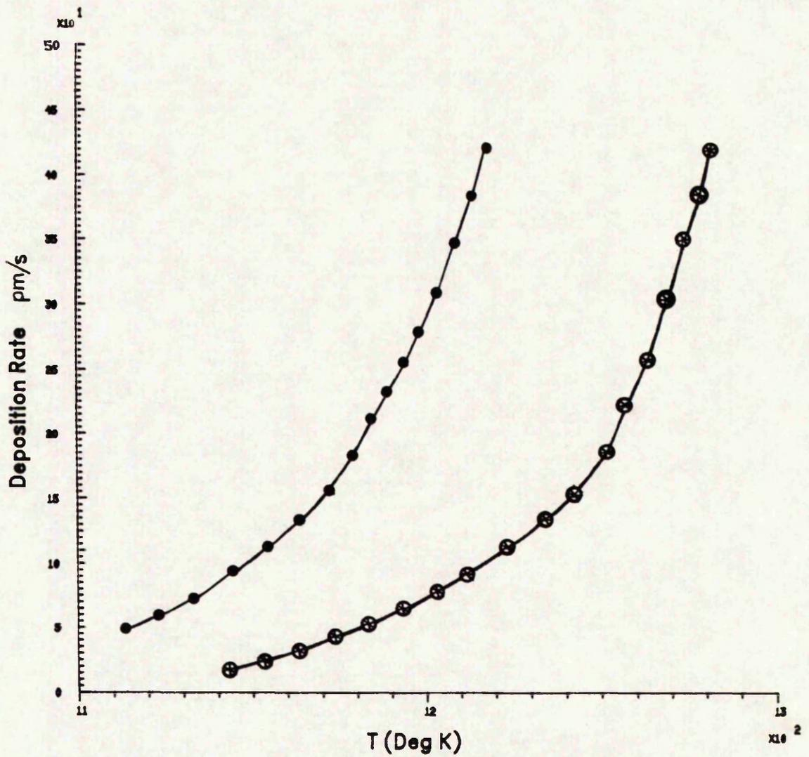
VARIATION OF THE DEPOSITION RATE WITH THE ABSOLUTE TEMPERATURE FOR ZnS (●) AND ZnSe (⊗).
