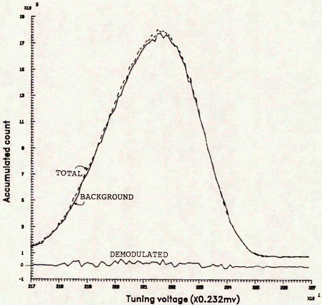
N2+ DIRECT, BACKGROUND AND DEMODULATED PEAK PROFILE AT 800 DEGREES CELSIUS AND 2MA EMISSION CURRENT
