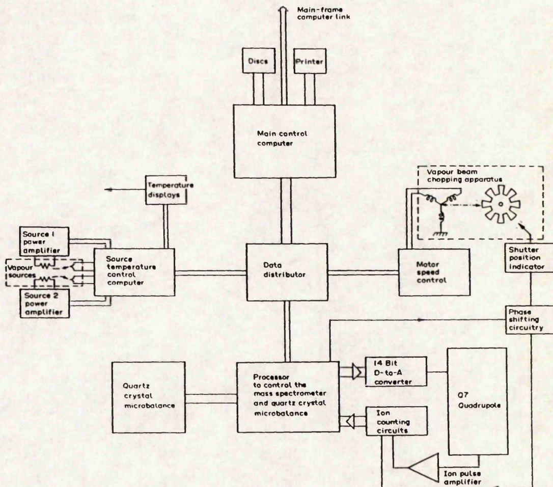
Figure 2. Schematic diagram of the electronic system used to control film deposition.
