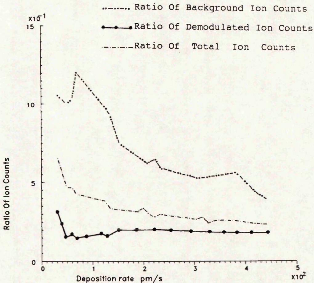
VARIATION OF THE RATIO OF BACKGROUND, DEMODULATED AND TOTAL ION COUNTS FOR  $Zn^+(m/e=33)$  OVER  $Zn^+(m/e=64)$  WITH THE DEPOSITION RATE (AT 200  $\mu A$  Emmission Current)
