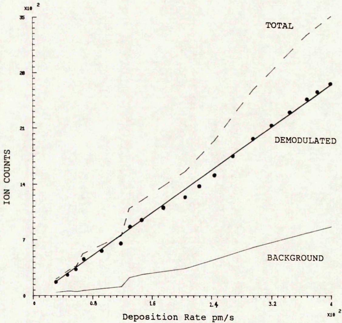
VARIATION OF  $\text{Se}^+$  ( $m/e=78$ ) ION COUNTS WITH THE TOTAL DEPOSITION RATE
