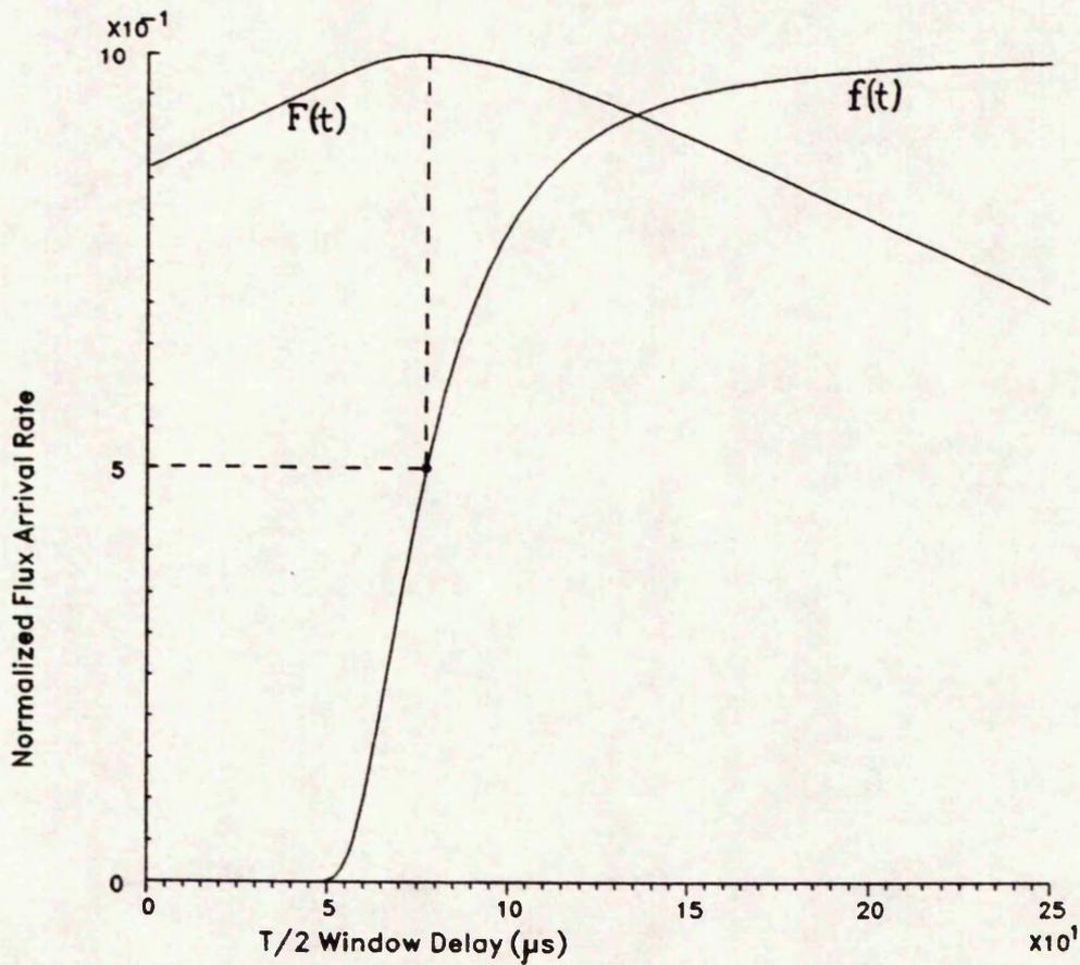
CALCULATED INTEGRATED ION ARRIVAL CURVE FROM THE ION ARRIVAL DATA FOR  $\text{Se}^+$  AT  $F_m=1\text{Khz}$ , 900 CELSIUS
