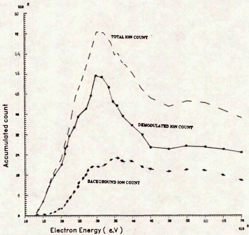
APPEARANCE POTENTIAL CURVES AT  $m/e=34$  DURING THE EVAPORATION OF ZnS AT 1000 °C
