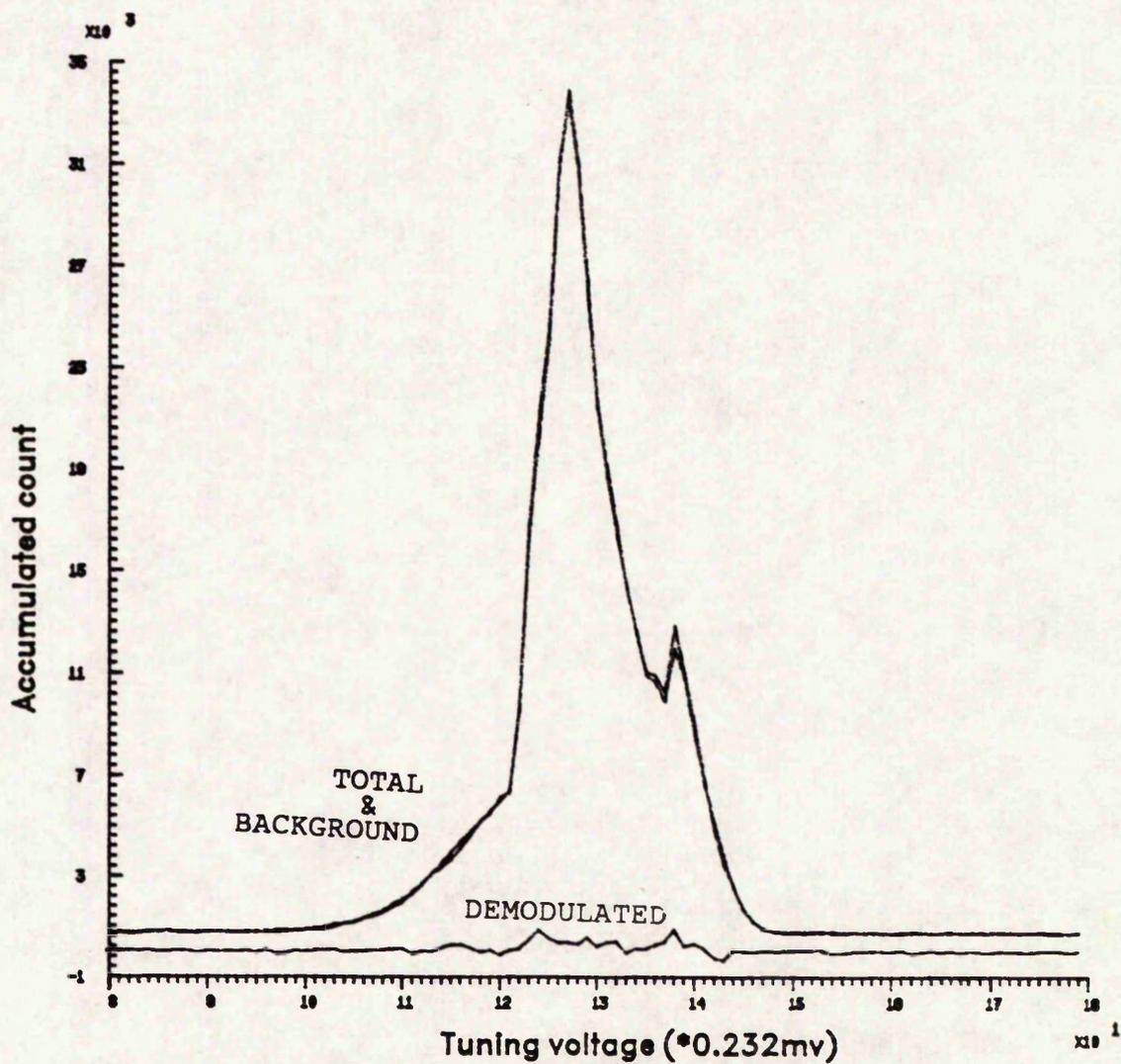
H<sub>2</sub><sup>+</sup> DIRECT BACKGROUND AND DEMODULATED PEAK PROFILE AT 800 DEGREES CELSIUS AND 2MA EMISSION CURRENT
