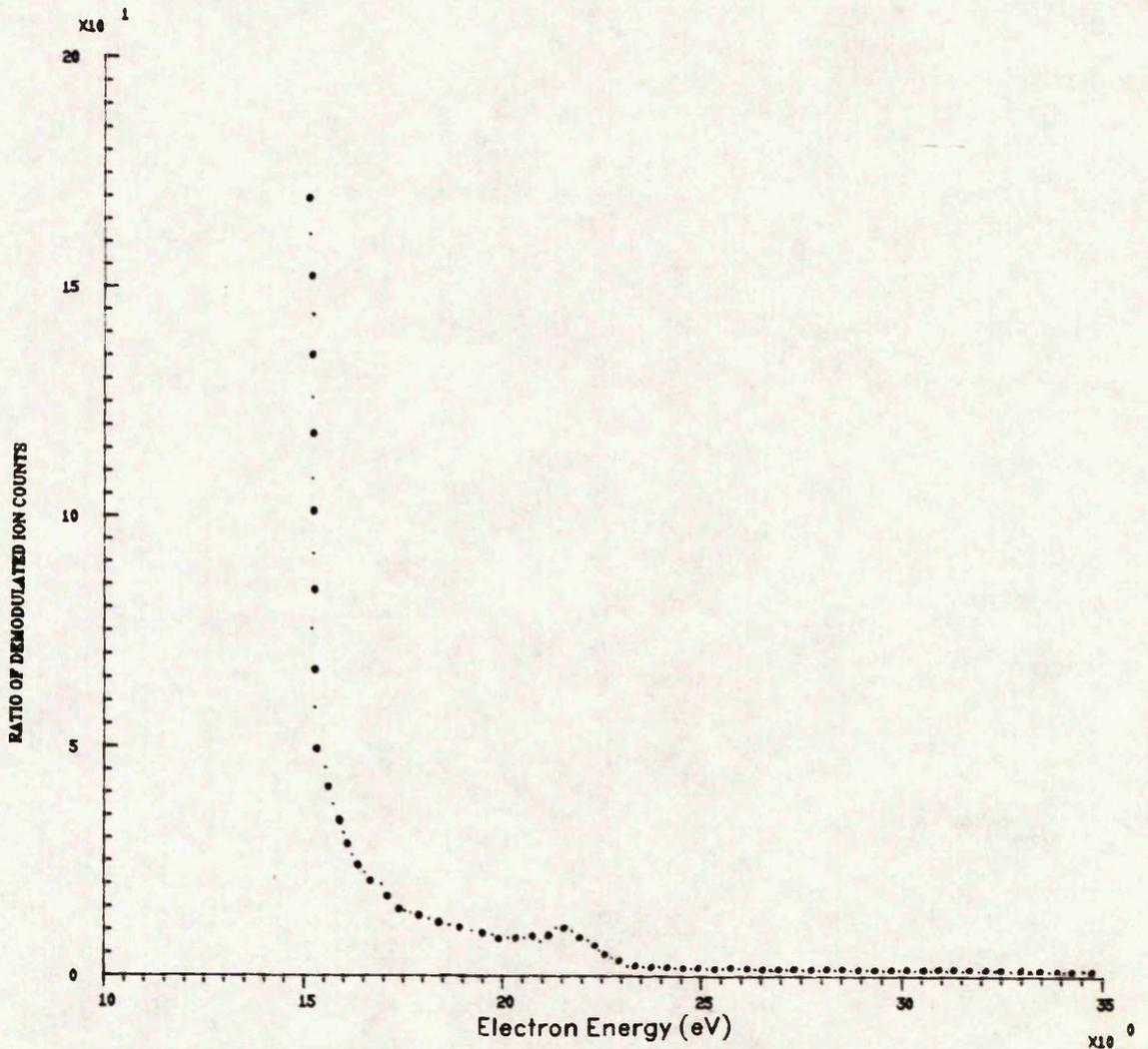
VARIATION OF THE RATIO BETWEEN THE ION COUNT FOR S<sub>2</sub><sup>+</sup> (m/e=64) AND S<sup>+</sup> (m/e=32) WITH THE ELECTRON ENERGY AT 1000 CELSIUS
