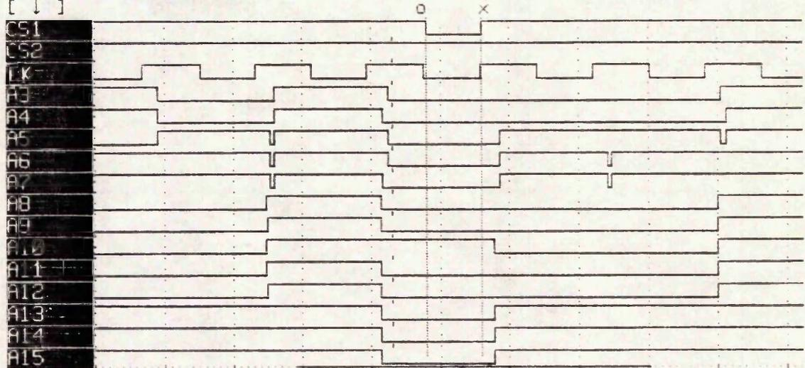
TIMING DIAGRAM OBTAINED BY DECODING ADDRESS 0400HEX
