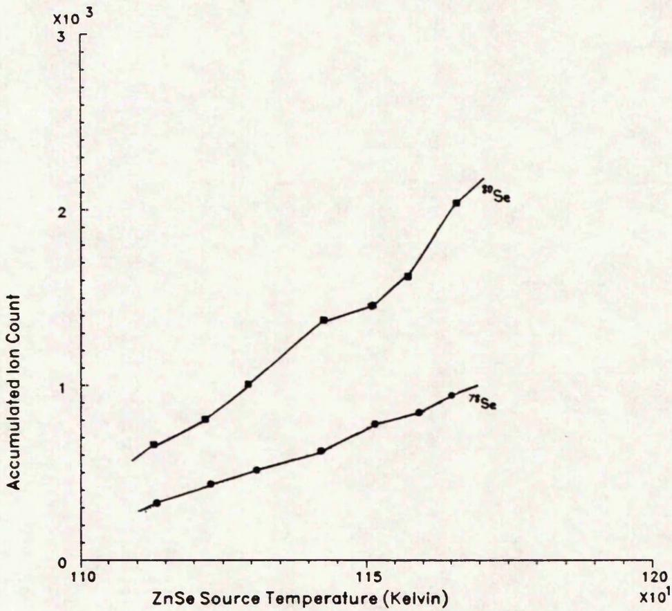
ION COUNTS VARIATION WITH THE ABSOLUTE SOURCE TEMPERATURE AT  $m/e=78$  AND  $80$  DURING THE DEPOSITION ZINC SULPHOSELENIDE
