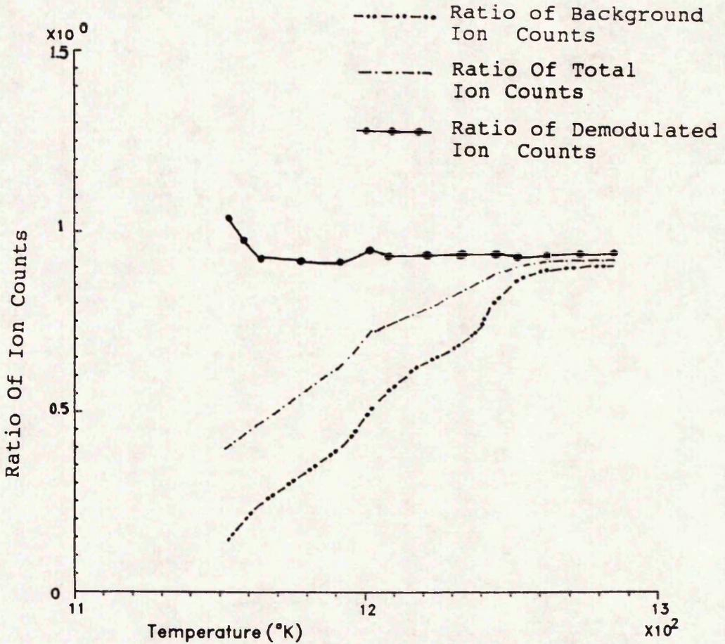
VARIATION OF THE RATIO BETWEEN  $\text{S}^{2+}(64)$  AND  $\text{Zn}^{+}(64)$  NUMBER DENSITIES WITH THE ABSOLUTE SOURCE TEMPERATURE
