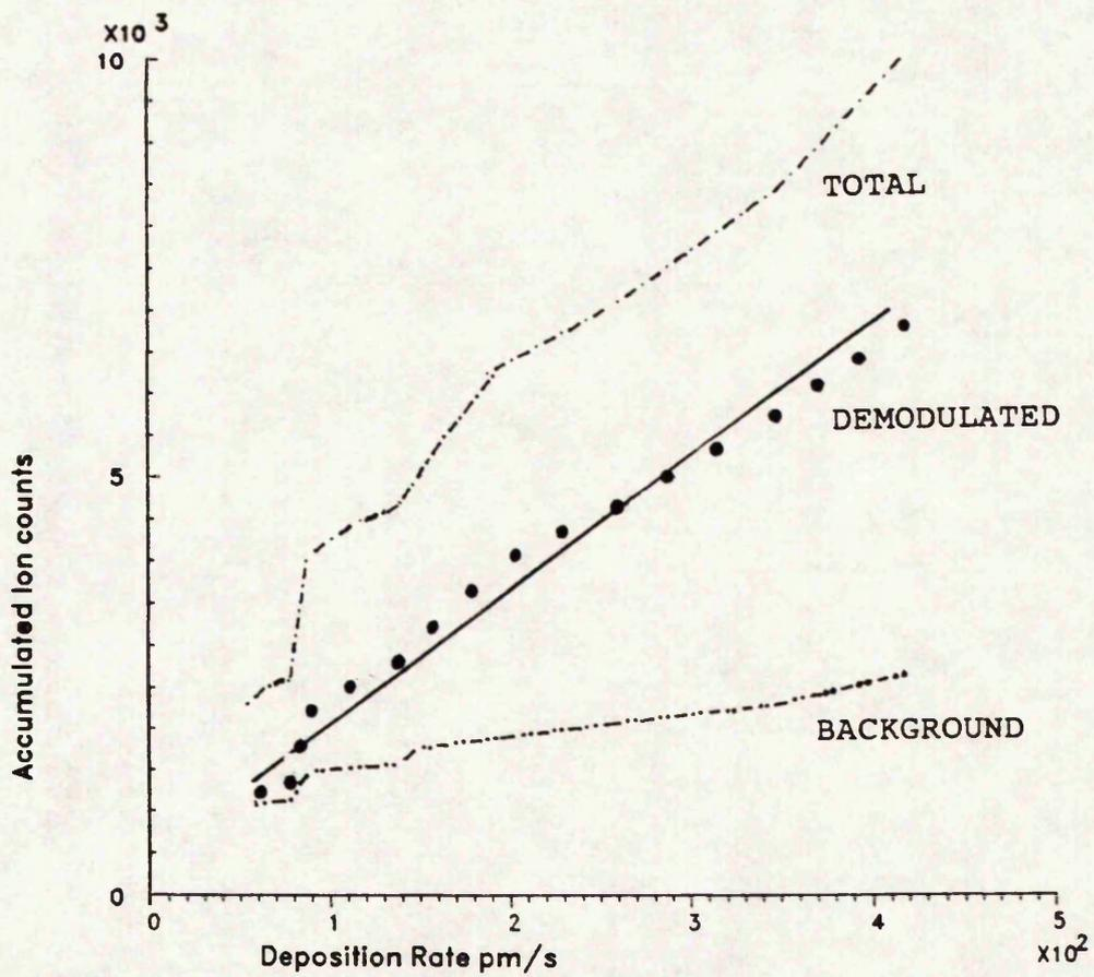
VARIATION OF  $Zn^+$  ( $m/e=64$ ) ION COUNTS WITH THE TOTAL DEPOSITION RATE
