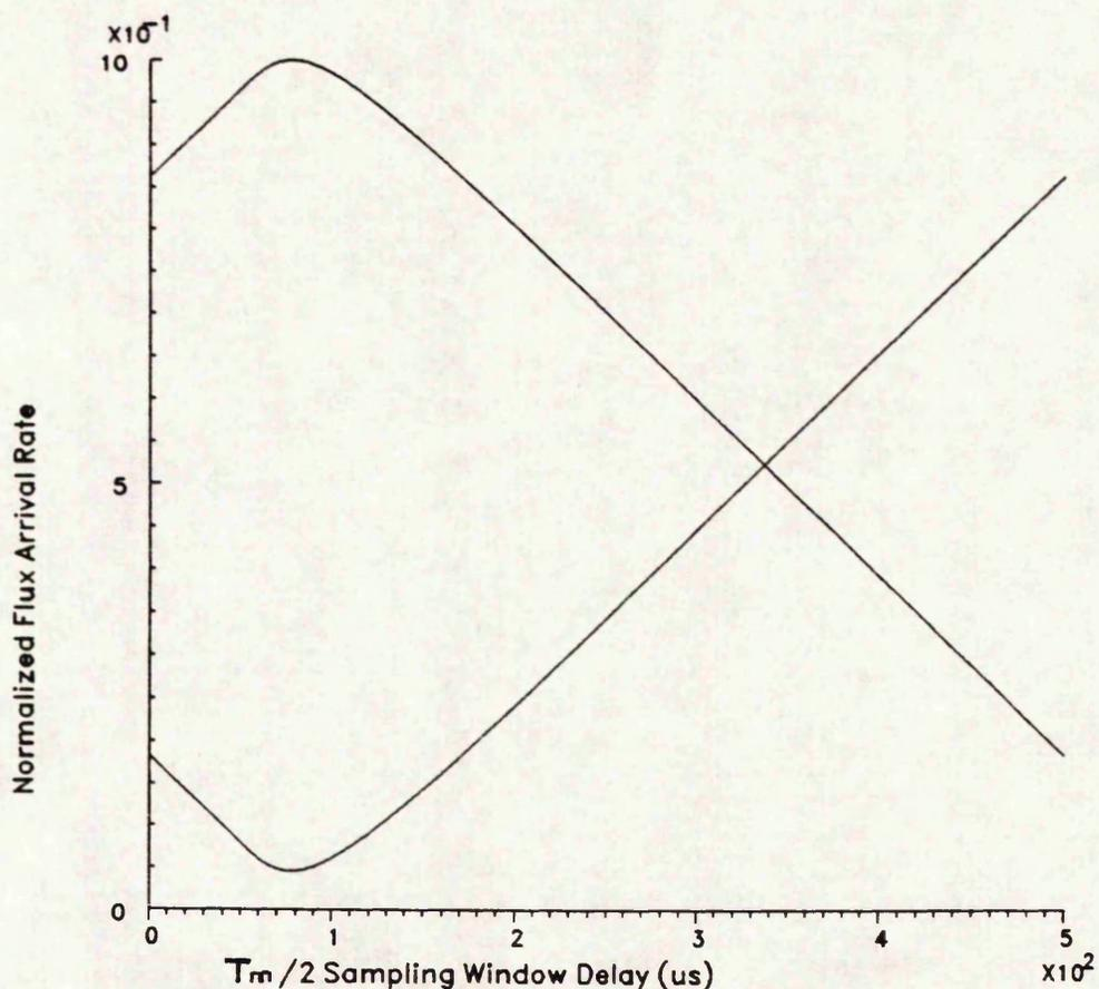
AN ALTERNATIVE REPRESENTATION FOR THE CALCULATED INTEGRATED ION ARRIVAL CURVE FOR  $\text{Se}^+$  AT  $F_m=1\text{Khz}$ , 900 CELSIUS
