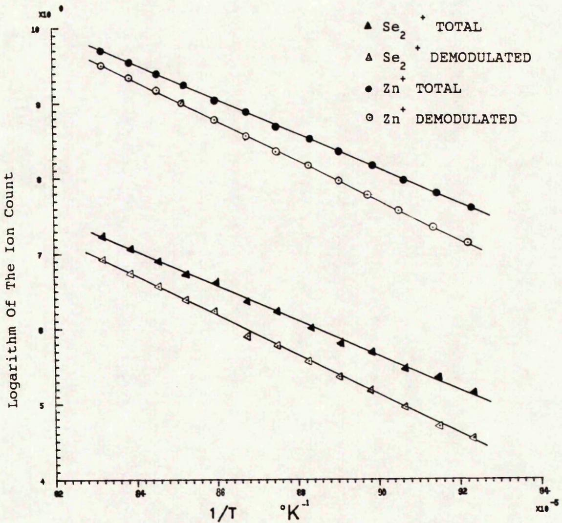
VARIATION OF THE LOGARITHM OF THE ION COUNT FOR  $\text{Zn}^+$  ( $m/e=64$ ) AND  $\text{Se}_2^+$  ( $m/e=160$ ) WITH THE INVERSE OF THE ABSOLUTE SOURCE TEMPERATURE
