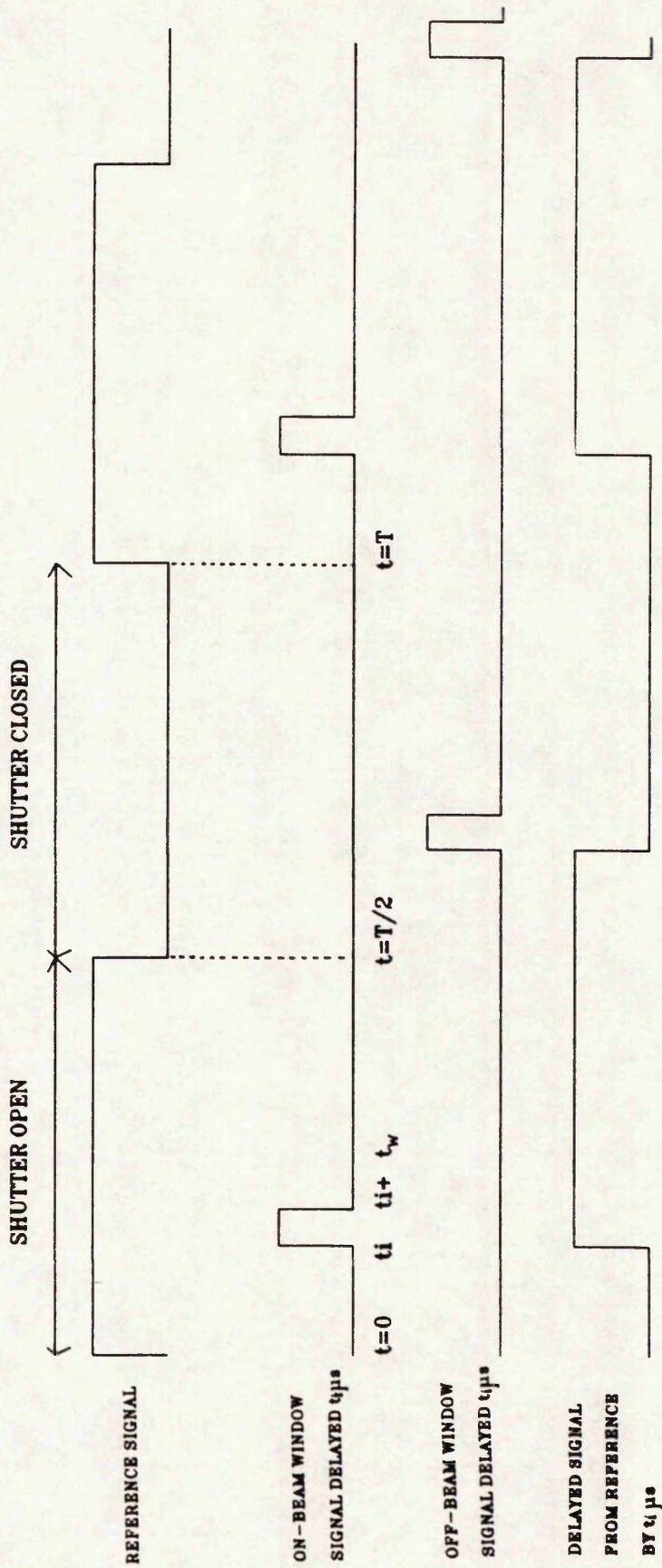
GATING WAVEFORMS USED FOR COUNTING THE EVAPORANT STREAM ION PULSES
