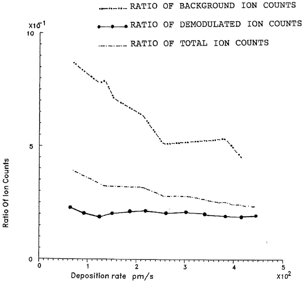
VARIATION OF THE RATIO OF BACKGROUND, DEMODULATED AND TOTAL ION COUNTS FOR  $\text{Se}^+$  ( $m/e=80$ ) OVER  $\text{Zn}^+$  ( $m/e=64$ ) WITH THE DEPOSITION RATE
