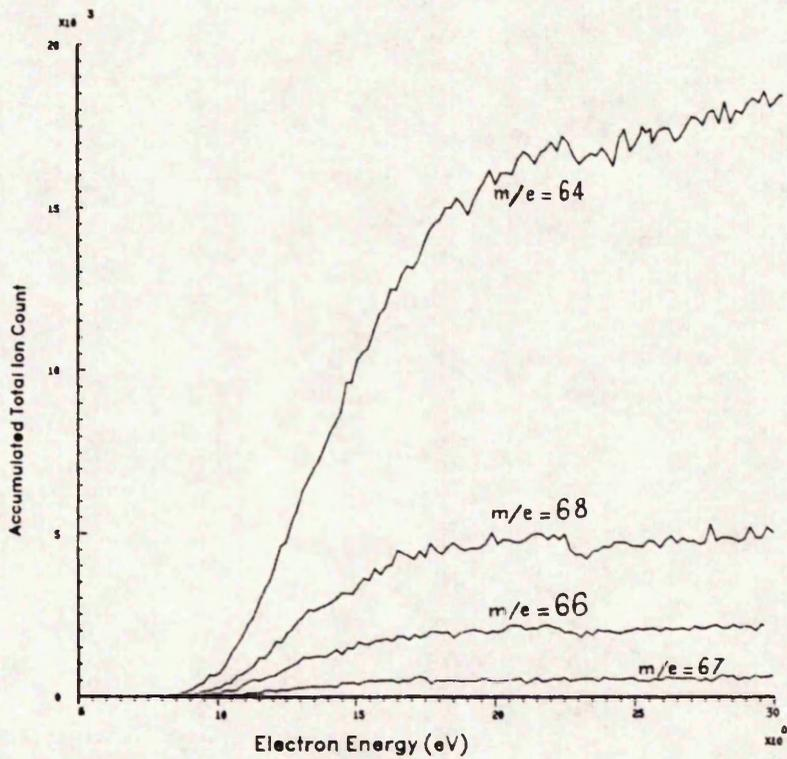
APPEARANCE POTENTIAL CURVES AT  $m/e=64, 66, 67$  AND  $68$  DURING THE EVAPORATION OF ZnS AT 915 °C
