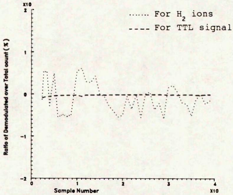
RATIO OF DEMODULATED OVER TOTAL ION COUNTS FOR  $H_2^+$  IONS ( $m/e=2$ ) AND PULSES FROM A TTL SIGNAL GENERATOR
