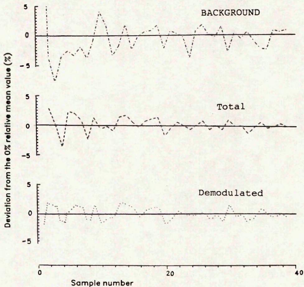
RELATIVE DEVIATION FROM THE MEAN VALUE FOR THE BACKGROUND, TOTAL AND DEMODULATED ION COUNTS FOR SELENIUM AT  $m/e=80$
