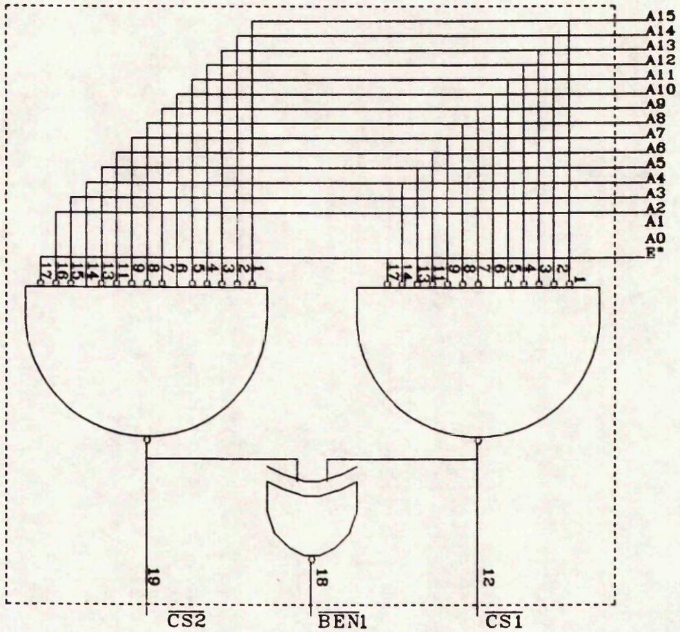
Logic Equivalent circuit to the PAL Used.
