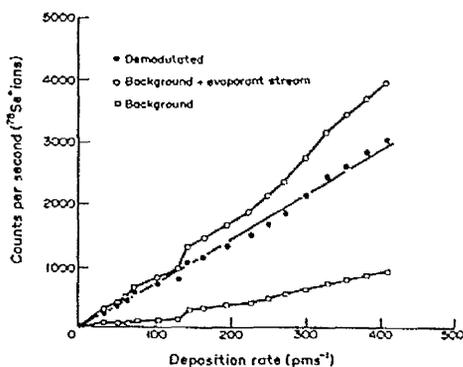
Figure 3. Particle count vs deposition rate for ZnSe.
