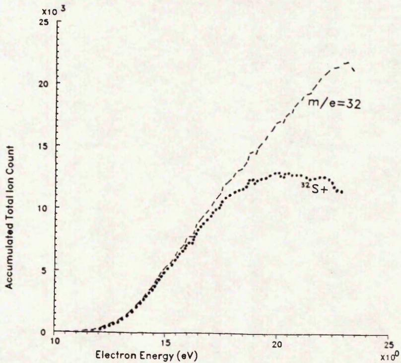
COMPARISON BETWEEN THE CALCULATED APPEARANCE POTENTIAL CURVE FOR  $S^+$  AND THAT AT  $m/e=32$  DURING THE EVAPORATION OF  $ZnS$
