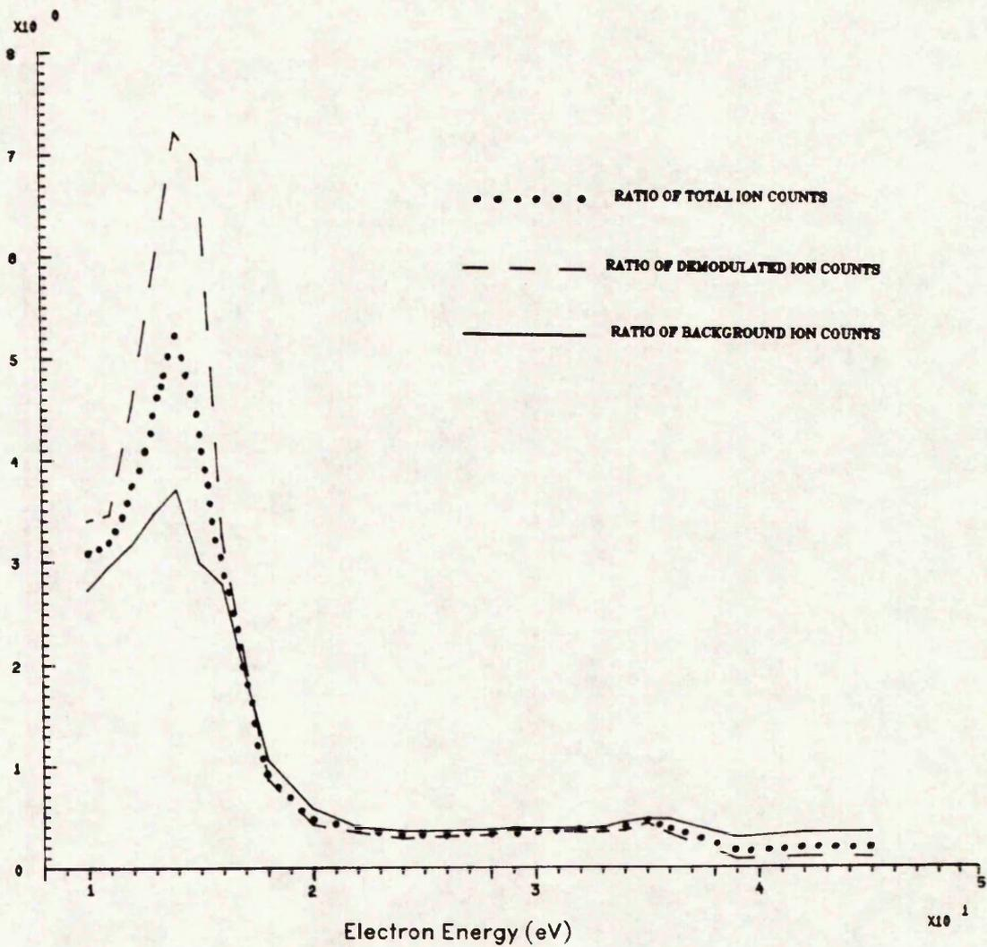
VARIATION OF THE RATIO BETWEEN THE ION COUNT FOR  $\text{Se}^{2+}$  ( $m/e=160$ ) AND  $\text{Se}^+$  ( $m/e=80$ ) WITH THE ELECTRON ENERGY AT 900 CELSIUS
