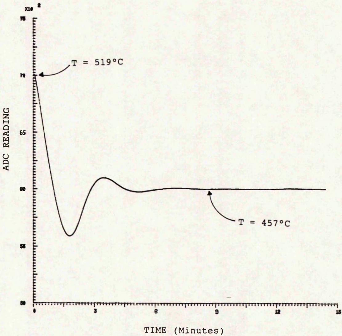
CURVE FOR THE CONVERGENCE OF THE ZnS SOURCE TEMPERATURE CONTROLLER TO A COMPUTED TEMPERATURE SET-POINT
