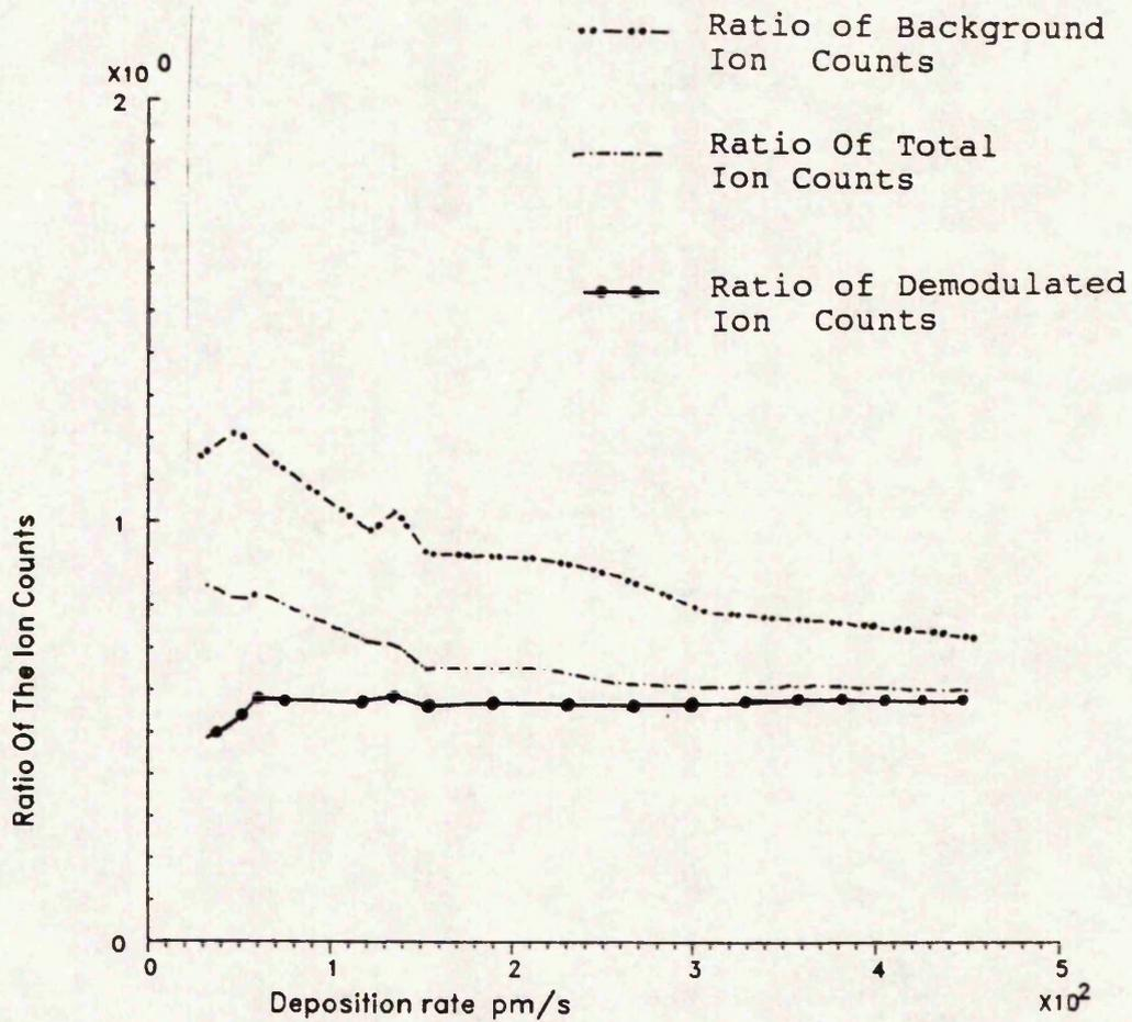
VARIATION OF THE RATIOS OF BACKGROUND, DEMODULATED AND TOTAL ION COUNTS FOR  $Zn^+$  ( $m/e=66$ ) OVER  $Zn^+$  ( $m/e=64$ ) WITH THE DEPOSITION RATE
