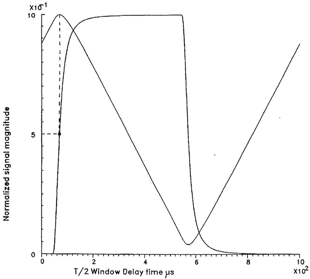
CALCULATED INTEGRATED ION ARRIVAL CURVE FOR  $\text{Zn}^+$
