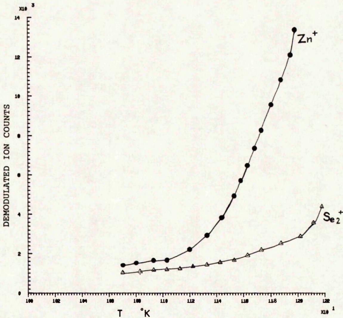
GRAPH OF  $\text{Se}_2^+$  AND  $\text{Zn}^+$  MEASURED NUMBER DENSITIES vs THE ABSOLUTE TEMPERATURE OF THE SOURCE
