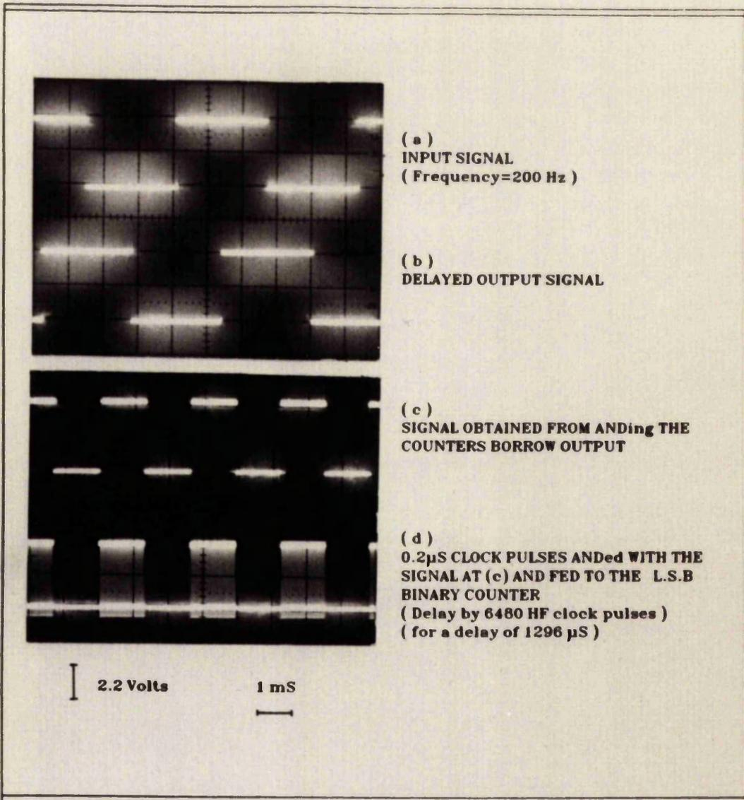
DIAGRAM SHOWING THE OSCILLOSCOPE TRACES OF THE SIGNALS
