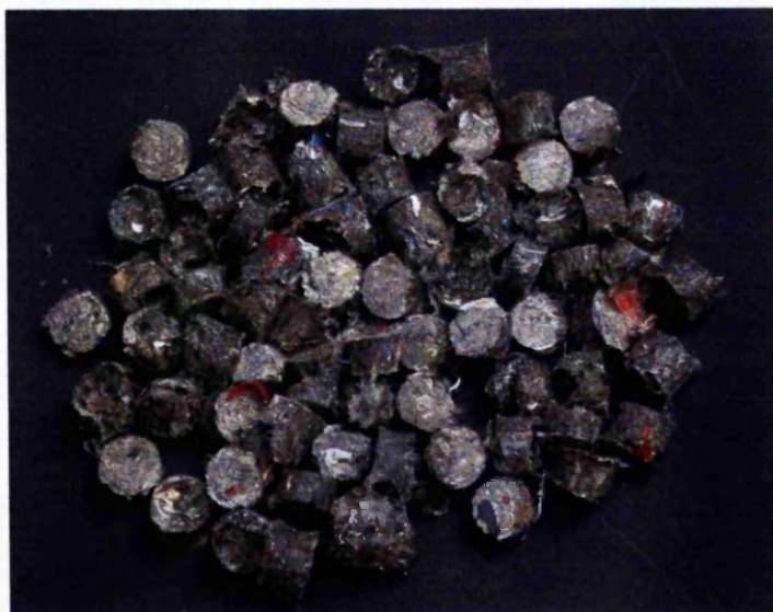
Figure 7. 2 A typical sample of the dRDF after preparation (approximately 10 mm lengths)
