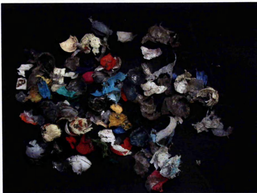
Figure 2. 6 Plastic materials removed from dRDF pellets.
