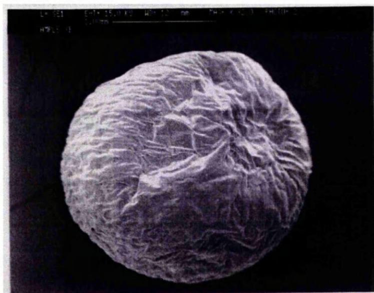
Figure 3.15 SEM of whole calcium alginate bead containing riboflavin showing external morphology (x 32.0).
