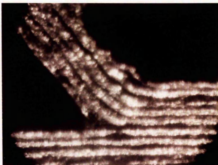
U = 17.3 \text{ m/min.} , t_1 = 0.3556 \text{ mm} , \alpha = 41^\circ , TOOL- HSS
