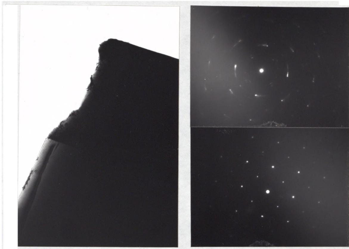
Figure 7.18 TEM micrograph of epitaxial ZnSe (top of picture) on GaAs substrate.
