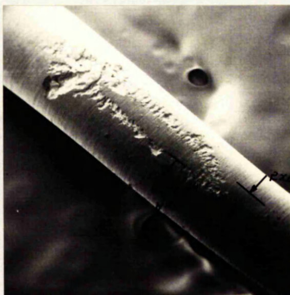
FIG. 6.3 SCANNING ELECTRON MICROGRAPH OF EROSION CRATERS
