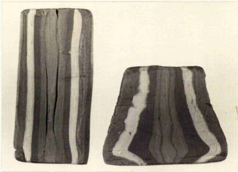
FIG. 3.7 SECTIONED PLASTICINE PROJECTILE (BEFORE AND AFTER IMPACT)
