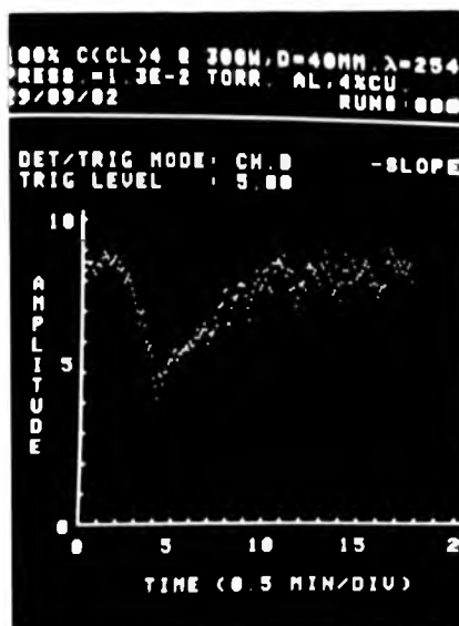
Fig.2.6.1 Reduction of optical emission at 255nm during RIE of Al/4% Cu.
