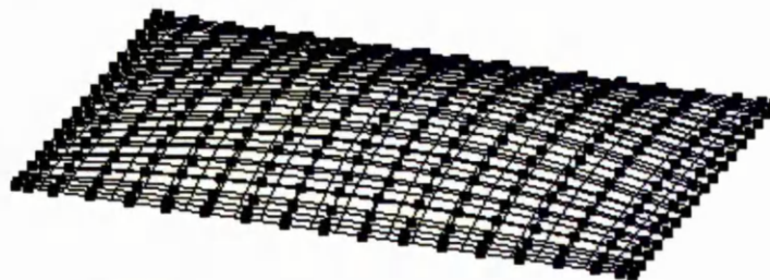
(b) The surface after knot refinement ( 19 \times 19 control points)
