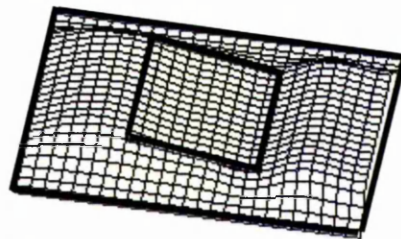
(b) The surface trimmed with the outer bounding box
