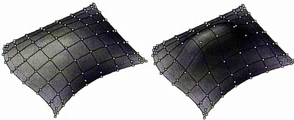
Figure 3.1: Direct control point manipulation
