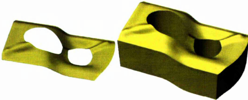
(b) The deformed trimmed surface and reconstructed B-rep model
