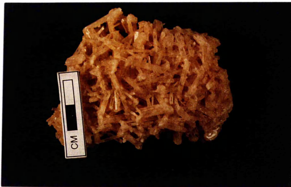
Plate (9.1) Celestite mineral, sample taken at 4.5 m, and found as geodic nodules. Benghazi Member, of the Ar Rajmah Formation. In Benghazi Cement Quarry.
