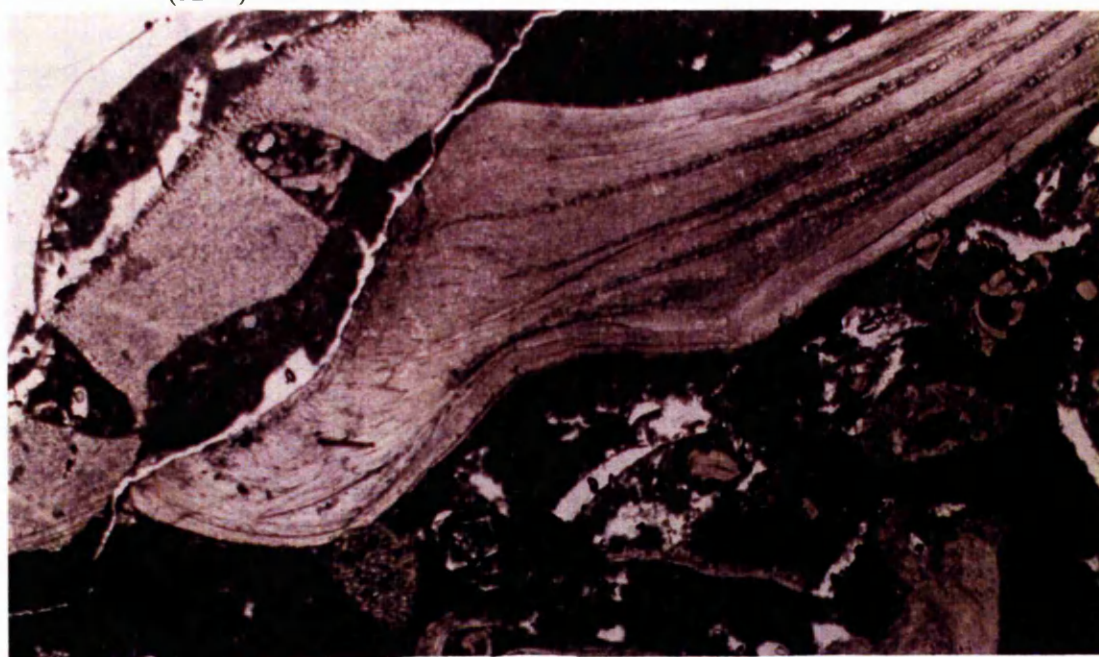
Plate (4.24) Large oyster fragments with foliated structure, and echinoderm fragments, Al Abra q Formation (A2), Deryanah Al Abyar road-cut. Field of view = 6 mm, (PPL).
