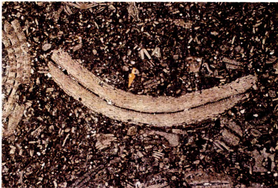
Plate (4.14) Longitudinal section of discocyclinid (arrowed) and Nummulites . The matrix is mainly micritic with many fragmented bioclasts (sample no. SUP). Field of view = 6mm, (PPL).
