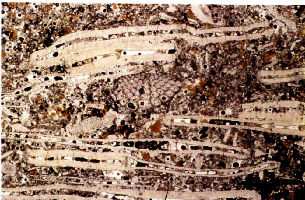
Plate (4.34) Transverse cross section of bryozoan with regular hexagonal shaped chambers or cellular structure, Al Faidiyah Formation (ULst.1). Field of view = 6 mm, (PPL).
