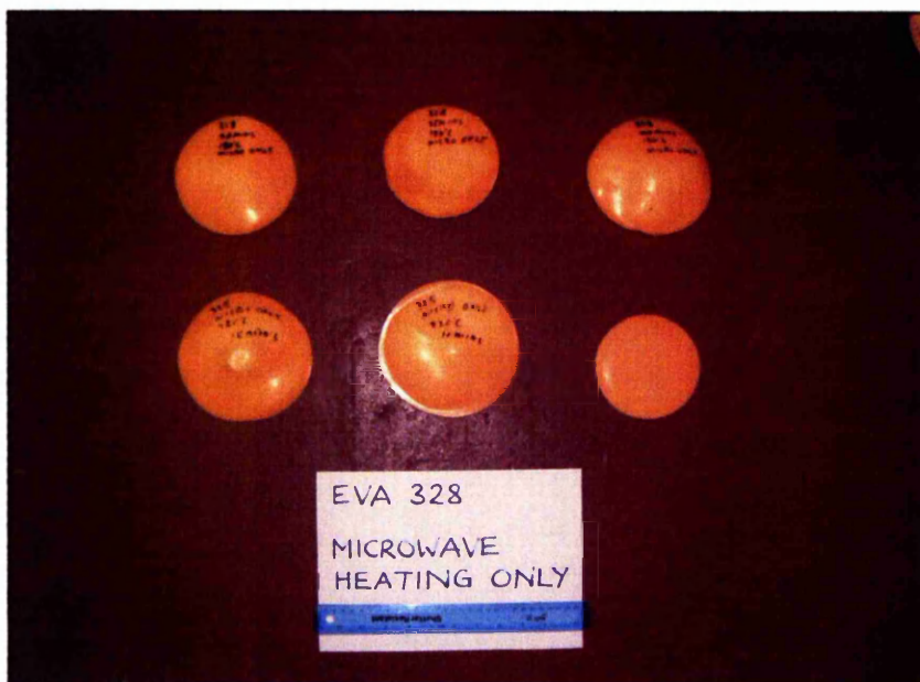
Figure 7.21: EVA 328 samples produced using microwave heating only, top left to bottom right, 180, 190, 200, 210, 220 °C microwave set point temperatures (bottom right unfoamed sample for comparison)
