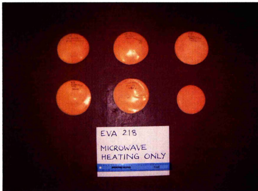
Figure 7.20: EVA 218 samples produced using microwave heating only, top left to bottom right, 180, 190, 200, 210, 220 °C microwave set point temperatures (bottom right unfoamed sample for comparison)
