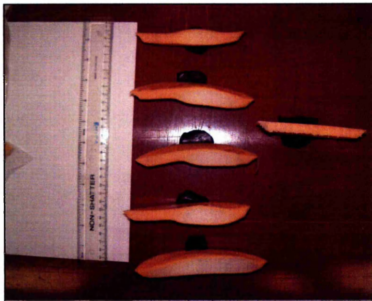
Figure 7.22: Cross sections of EVA 218 foams produced using microwave heating only (180, 190, 200, 210, 220 °C set point temperature top to bottom). A cross section of an unfoamed sample is shown on the right for comparison
