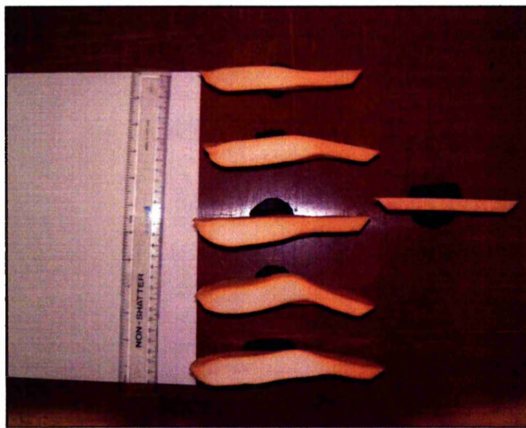
Figure 7.23: Cross sections of EVA 328 foams produced using microwave heating only (180, 190, 200, 210, 220 °C set point temperature top to bottom). A cross section of an unfoamed sample is shown on the right for comparison
