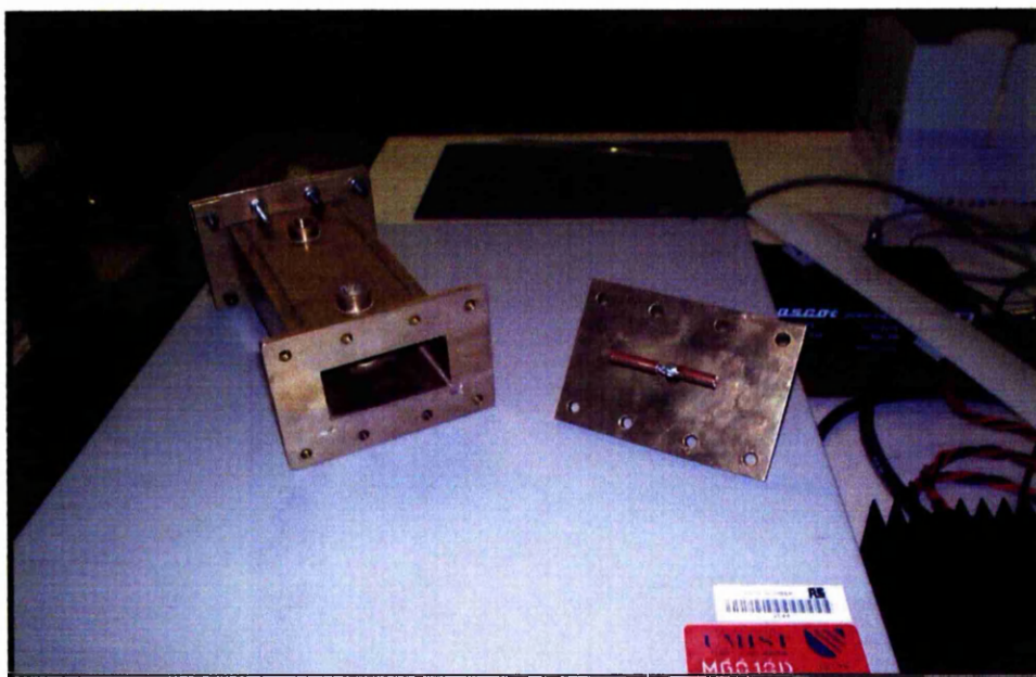
Figure 5.3: Rectangular brass waveguide applicator and antenna
