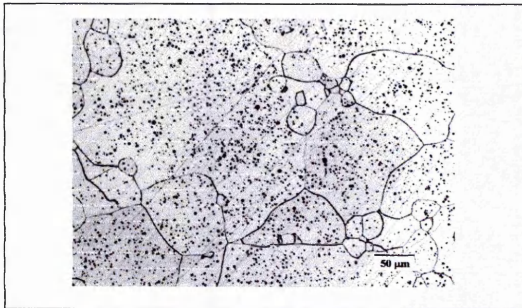
Figure 4.15 Optical micrograph of Mn-Zn ferrite with 0.4 wt% \text{HfO}_2 in combination with 0.02 wt% \text{SiO}_2 additions, (a) sample prepared by gel processing, (b) sample prepared by mixed oxides method (route 1), and (c) sample prepared by mixed oxides method (route 2).
