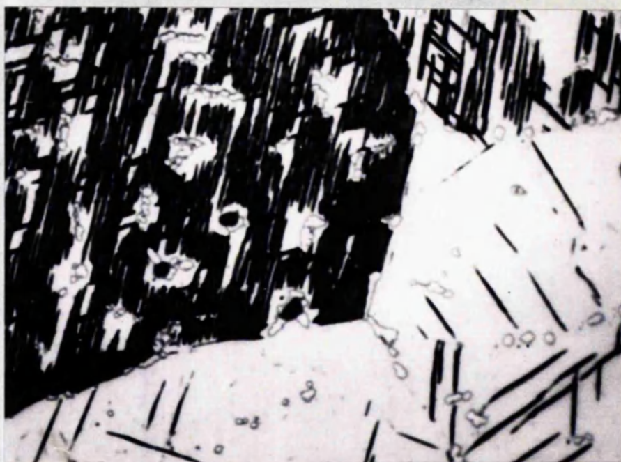
Plate 4. Fe-V, slow quench from 1250°C. x 400.
