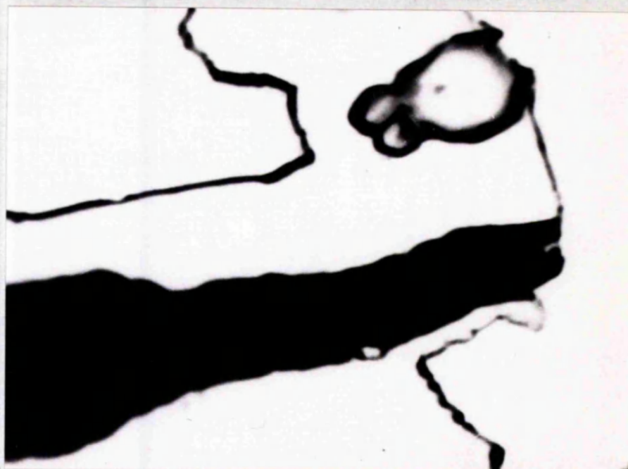
Plate 12. Fe-V-W, quenched from 1350°C and partially transformed at 760°C. x 400.
