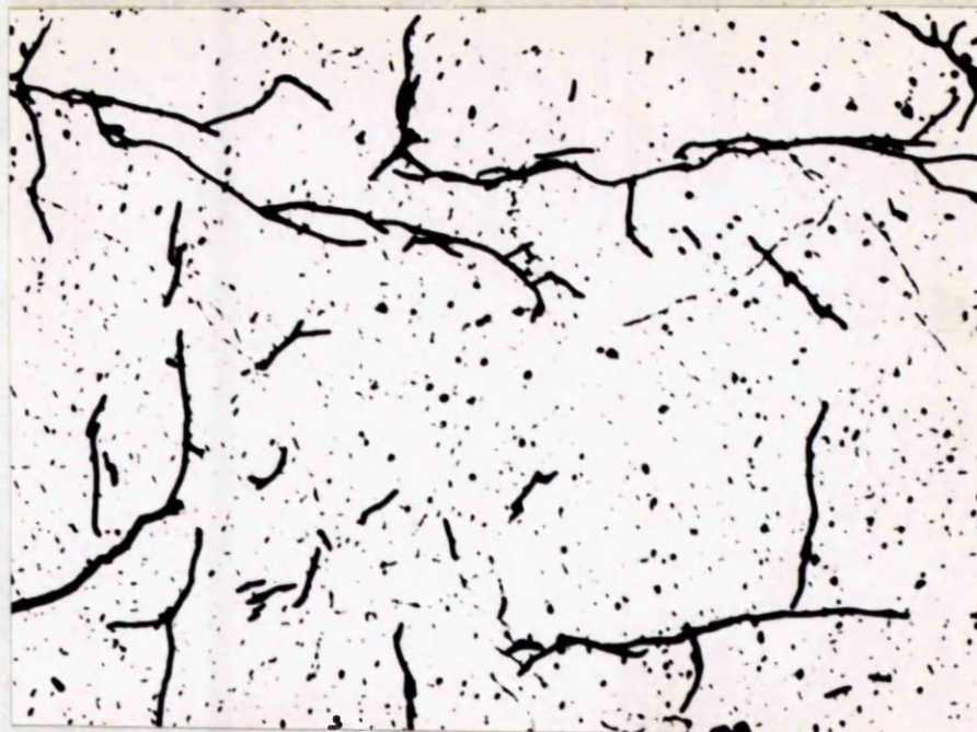
Plate 13. Fe-V, quenched from 1350°C and isothermally transformed at 850°C. x 25.
