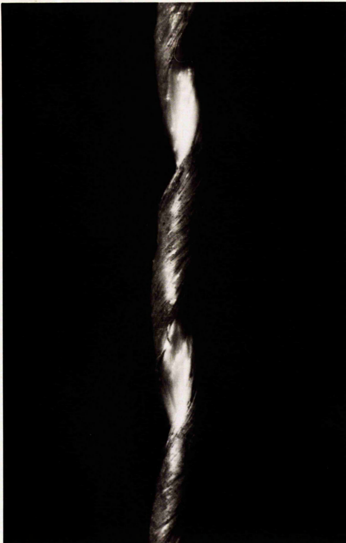
Fig. 4.32C. Tenasco 1650-750-12 yarn in the process of untwisting.
