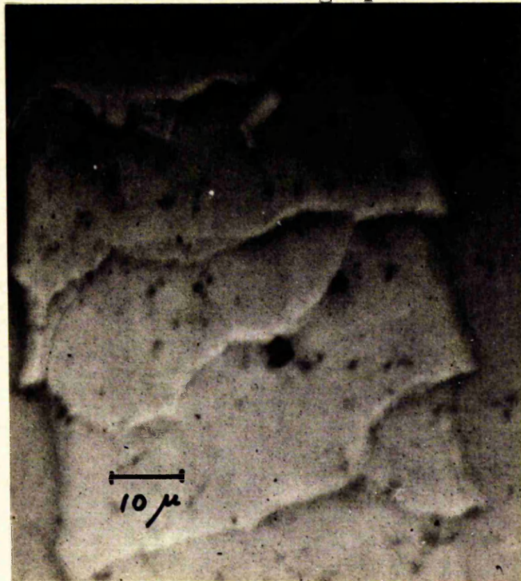
FIG.1. ELECTRON-MICROGRAPH OF WOOL FIBRE. 12,000 X.
