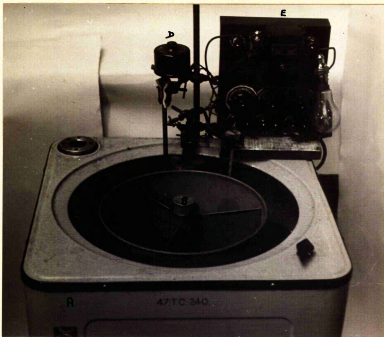
FIG. 28. THE NEW APPARATUS FOR FELTING TESTS.
