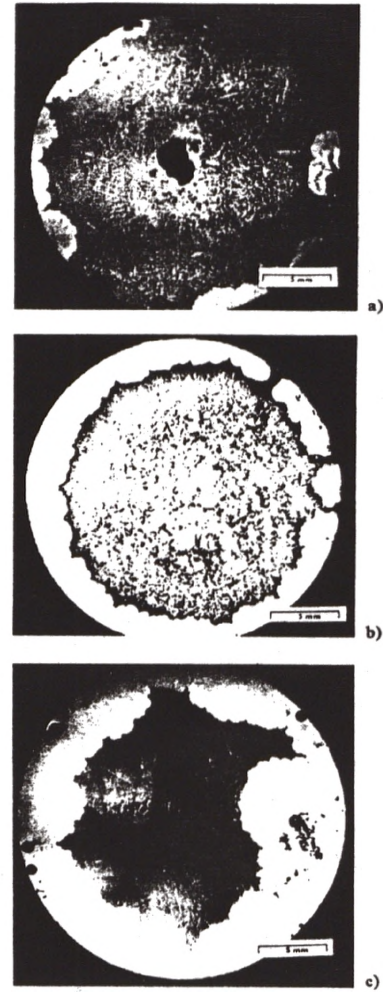
Figure 4: Quenched interfaces showing the development of a scalloped interface in strontium modified eutectic cooled at a rate of 4^{\circ}\text{C min}^{-1} . a) quenched after 2 minutes b) quenched after 4 minutes c) quenched after 6 minutes
