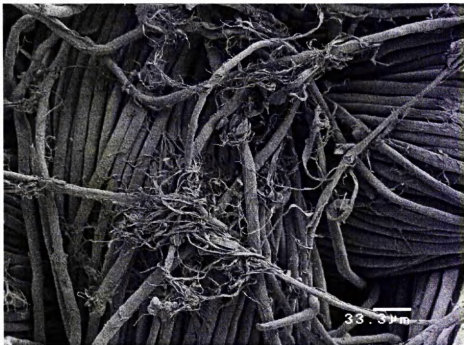
Picture 8.5 Untreated fabric after 15 laundering cycles
