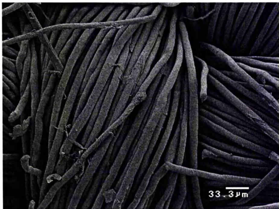
Picture 8.4 Fabric treated with 60 g/l Fixapret ECO after 10 laundering cycles
