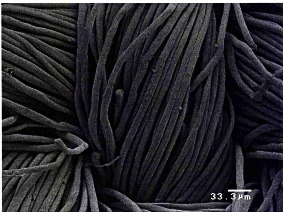
Picture 8.3 Fabric treated with 60 g/l Fixapret CP after 10 laundering cycles
