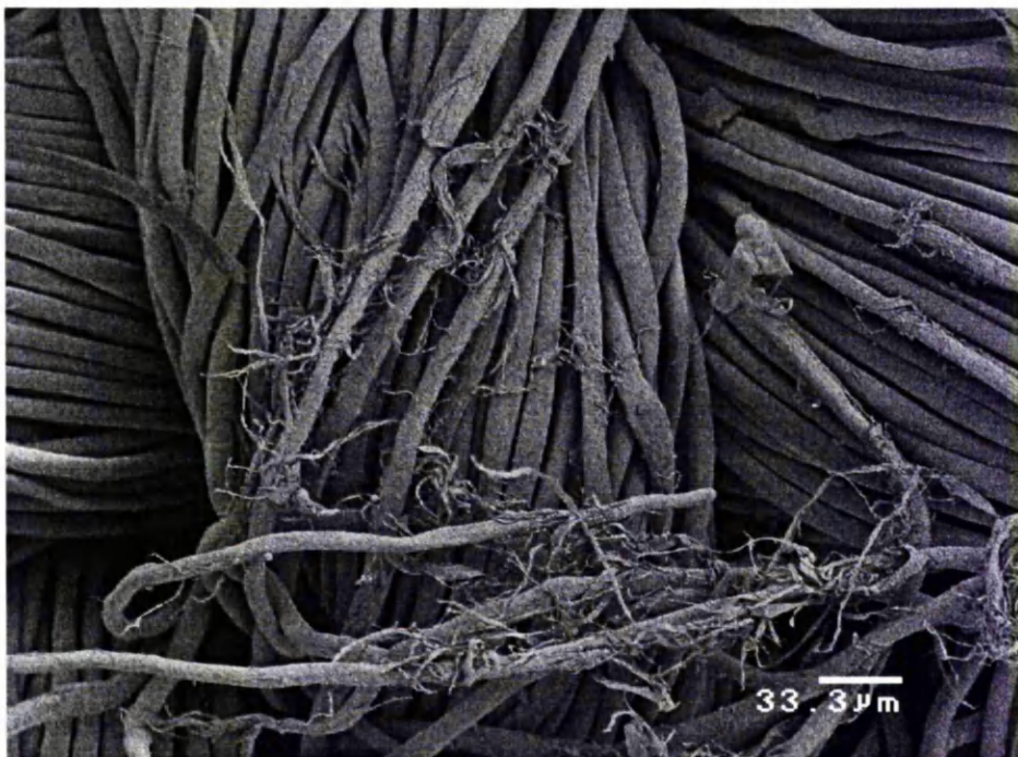
Picture 8.1 Untreated fabric after 10 laundering cycles
