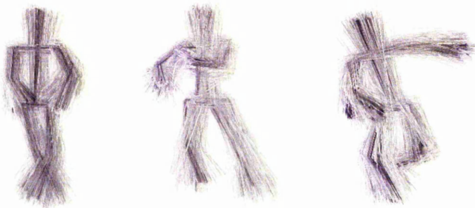
Figure 6.2: Sets of 1000 particles locally populating the parameter space of the model configurations, and weighted so as to estimate the distribution of the posterior .
