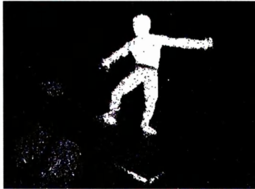
(b) Silhouette extraction using Grimson et al. [SG99]'s method (10 Gaussians per pixel).
