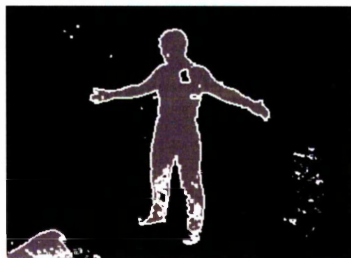
(e) Our algorithm classifying pixels with a 3 \times 3 window and handling of shadows.
