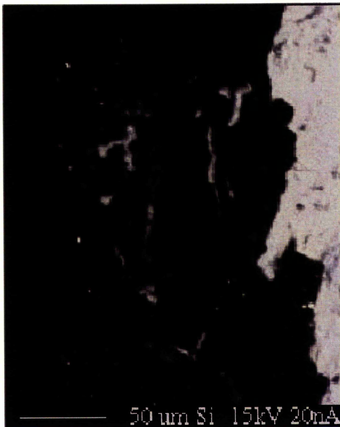
Figure 8.2c: Si element map of grain 1
