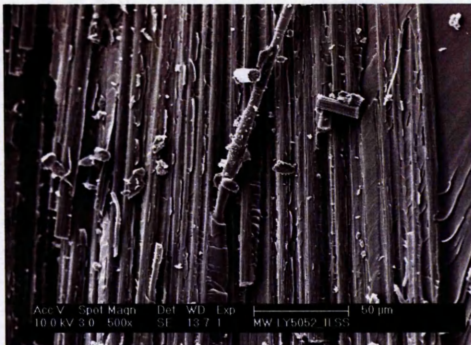
Figure 7.30: Fracture surface of microwave cured LY/HY5052/carbon composite subjected to interlaminar shear testing showing fibres coated with resin.
