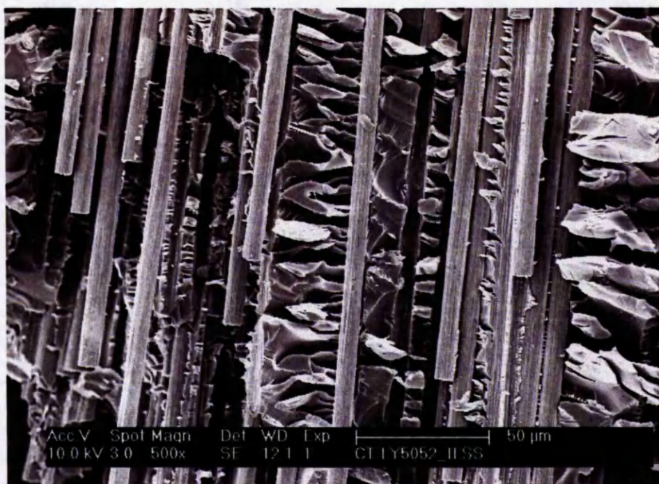
Figure 7.28: Fracture surface of conventionally cured LY/HY5052/carbon composite subjected to interlaminar shear testing showing clean fibres.
