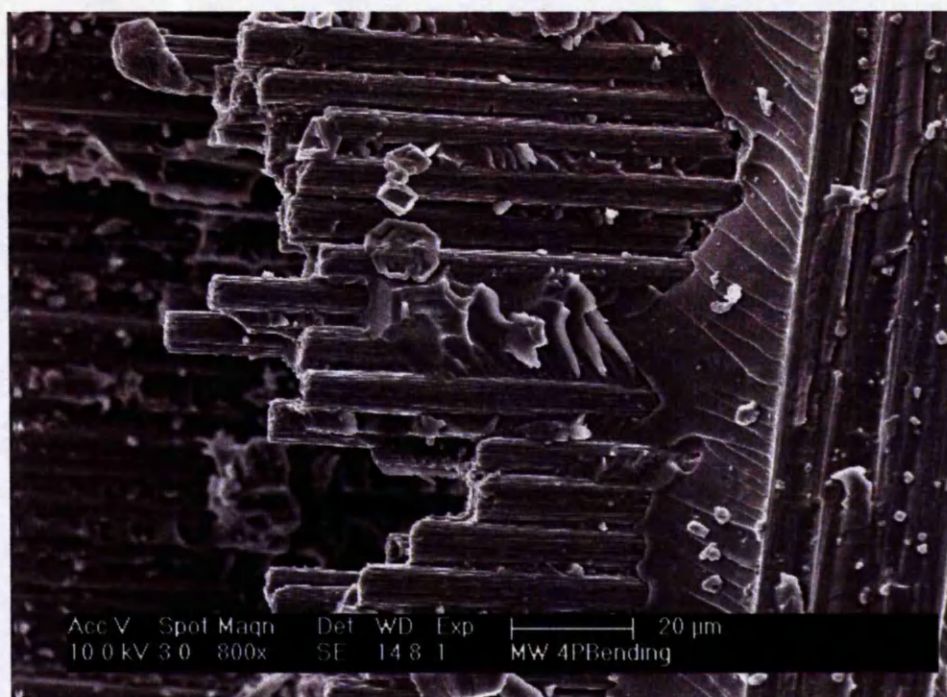
Figure 7.15: Fracture surface of microwave cured LY/HY5052/carbon composite subjected to four-point bending showing fibre breakage (left hand side) and fibre pull-out (right hand side).
