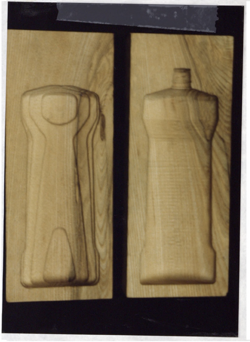
Picture 9. The wood blocks showing the results of the roughing and finishing operations for the bottle mould
