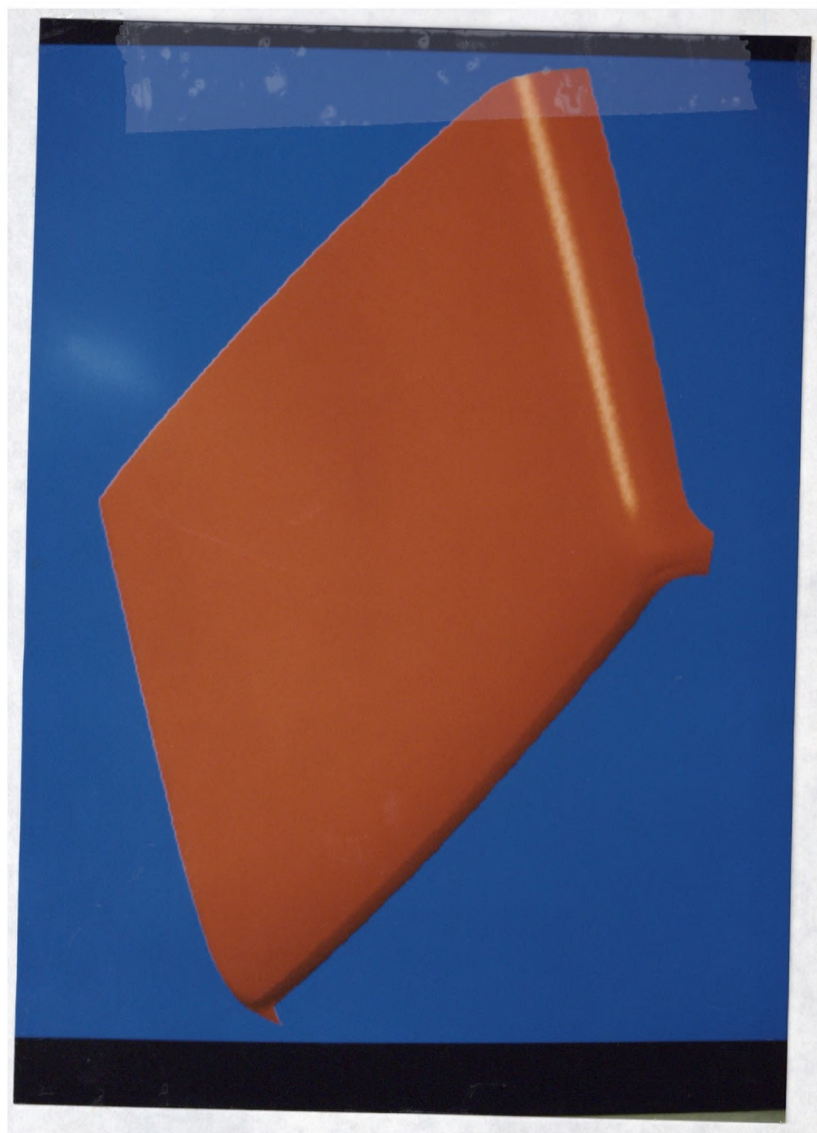
Picture 7 The model of the scaled cab roof supplied by LEYLAND-DAF (Overall scaler: 0.18)
