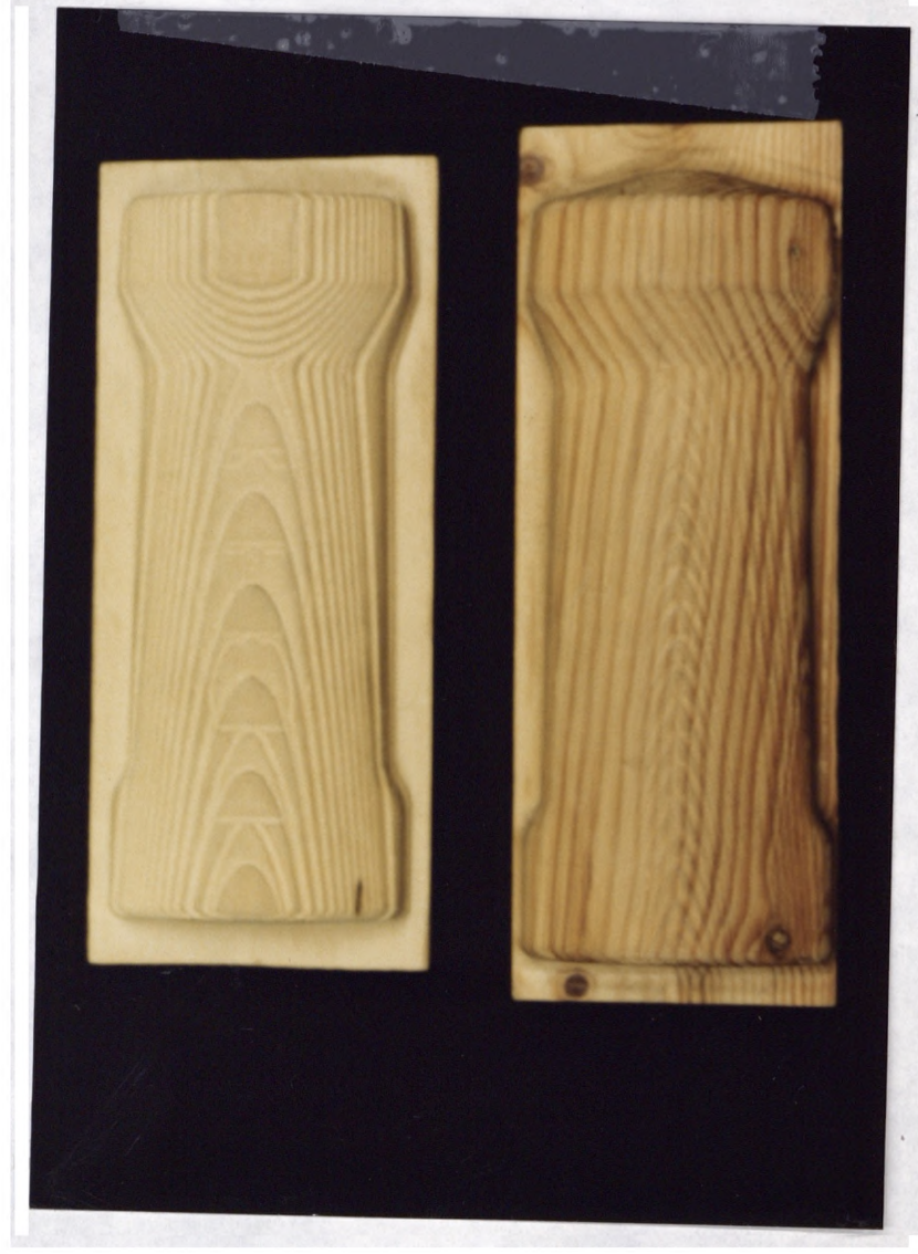
Picture 6 The bottle models machined using incorrect sizes of tools and in a wrong direction
