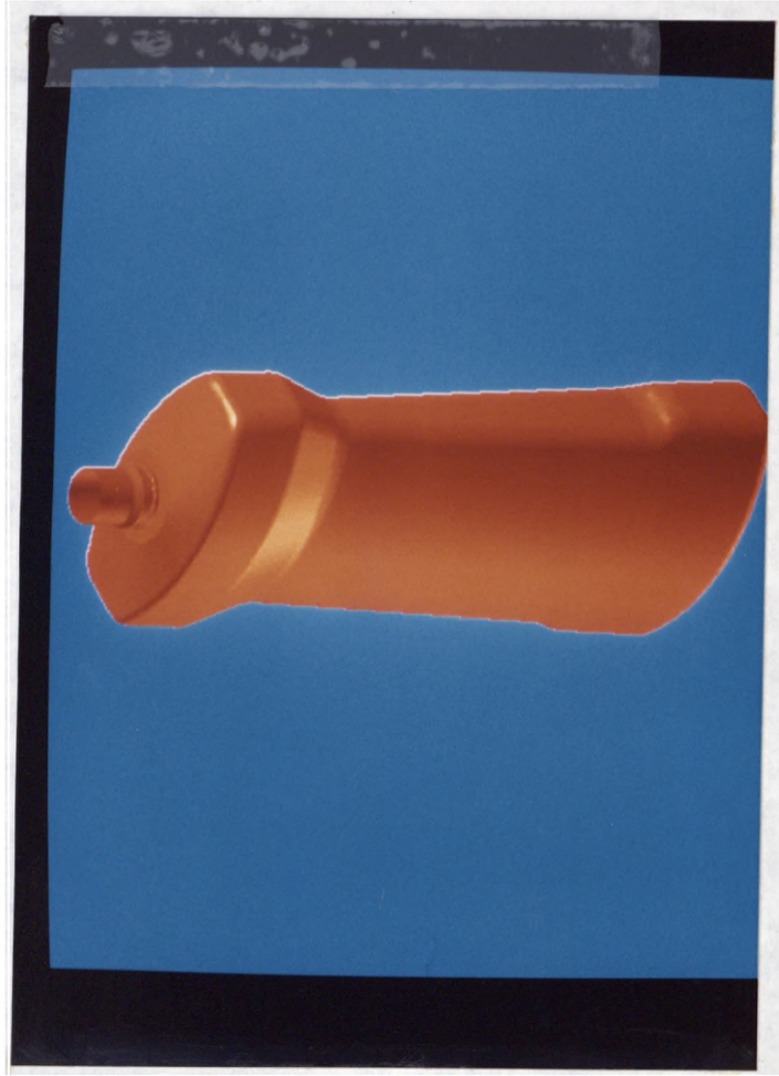
Picture 4. The model of the scaled bottle shown in Picture 3 (50% increase in volume, scaled in the cross sectional direction)
