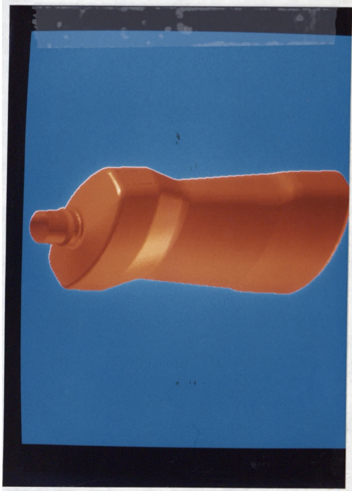
Picture 5. The model of the locally scaled bottle shown in Picture 3 (22.8% decrease in volume, scaled in the longitudinal direction)
