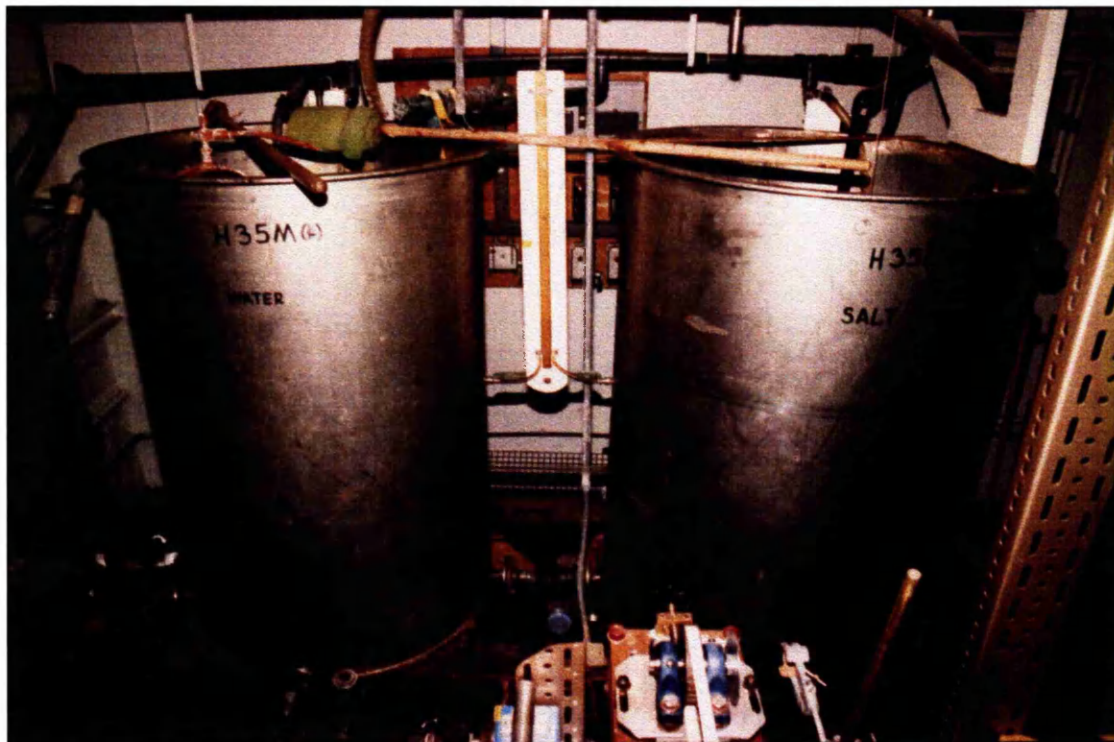
Figure 4.7 The two tanks used to contain fluid before filling the towing tank.
